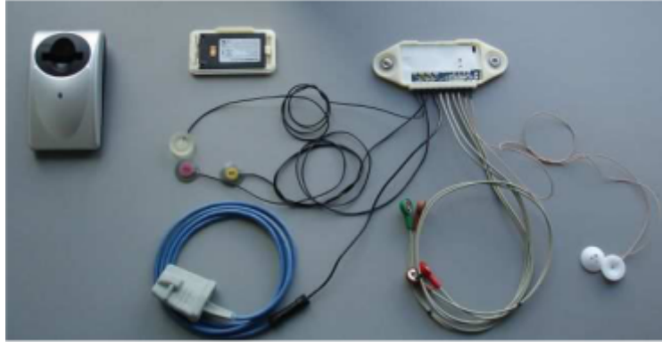
Figure 4.1: SENSATRON device and its components, central unit, battery and charger[5]
