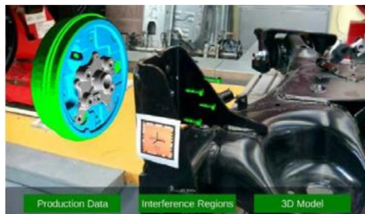
Figure 1.3. Digital components overlaid in real objects (Michalos et al., 2016).
