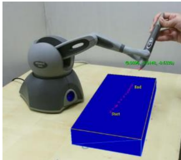
Figure 1.4. Path planning on the “augmented” workpiece (Li & Chu, 2016).
