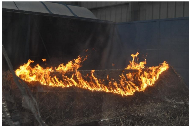
Figura 13 - Fenómeno Fire Channelling (2D12.27.20)
