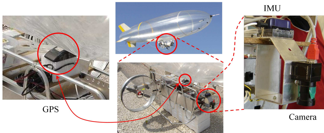
Figure 1.2: The DIVA airship, with details showing the vision-AHRS system and GPS receiver mounted on the gondola.
