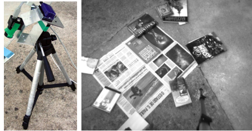
Figure 3.11: A tripod with a camera rigidly mounted with the AHRS, and an image example.
