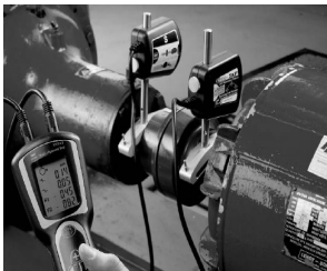
Fig. 2. Direct coupling and commercial equipment for shafts alignment.
