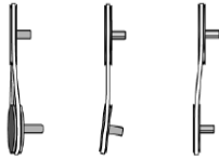
Fig. 9. Belt-pulley systems installation: (left) torsional misalignment; (center) angular misalignment; (right) parallel misalignment.
