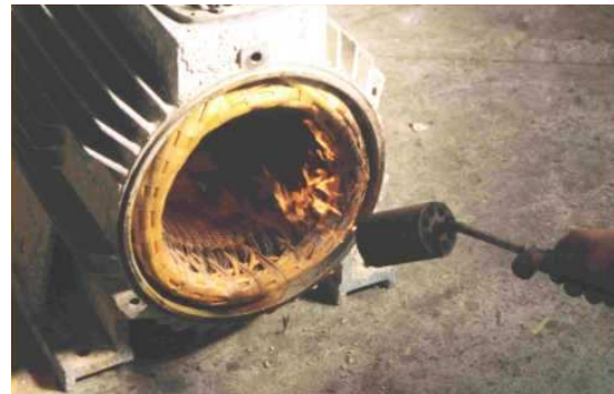
Fig. 27. Windings burning-out process using a gas torch.
