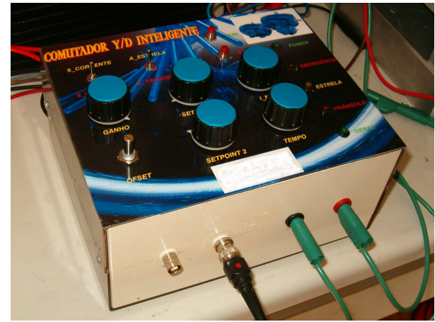
Fig. 2. First prototype of the electronic device ( Smart-Switch ) for automatic management of the stator winding connection as a function of the line current.
