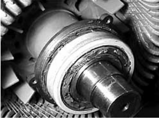
Fig. A5.38. Bearing with insulated outer ring installed in a rotor shaft.
