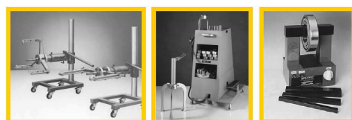
Fig. 29. Bearing handling: (left) manual bearing extractor open; (centre) hydraulic extractor; (right) induction bearing heater.
