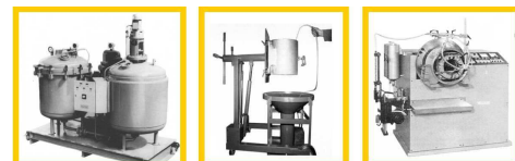
Fig. 30. Impregnation: (left) vacuum pressure or VPI; (centre) manual trickle; (right) automatic trickle.
