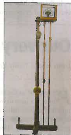
▲ Fig. 3: The Atwood Machine sent from London by John Magellan.
