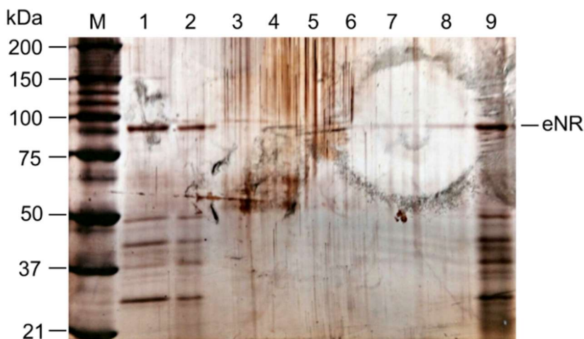
Figure 4.11. SDS-PAGE/silver staining of Aspergillus niger nitrate reductase. Lane M: molecular weight marker; Lane 1: eNR soluble; lane 2: eNR immobilized before any reaction; lane 3: non-bound protein after immobilization; lane 4: cycle 1; lane 5: cycle 2; lane 6: cycle 3; lane 7: cycle 4; lane 8: cycle 5; and lane 9: eNR immobilized after 5 reaction cycles.
