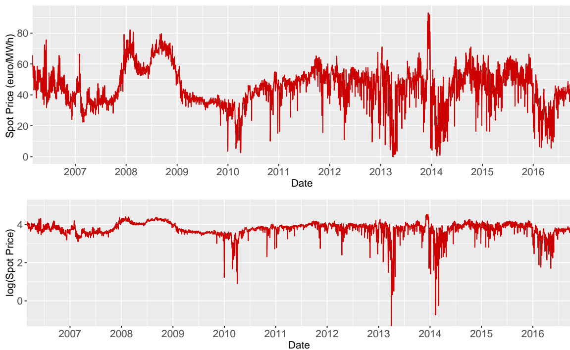
Fig. 7.1 Daily electricity prices (top), in units of €/MWh, and the logarithm of daily prices (bottom) traded for the day-ahead on MIBEL, over the time period of 1 March 2006 to 30 September 2016.
