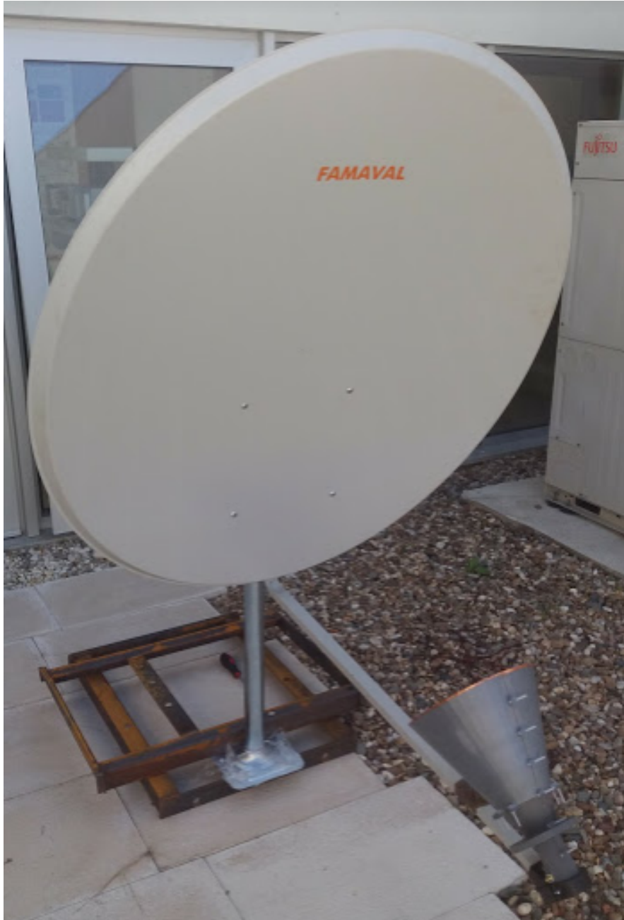
FIGURE 8.2: Emitter antenna and first parabolic reflector.
