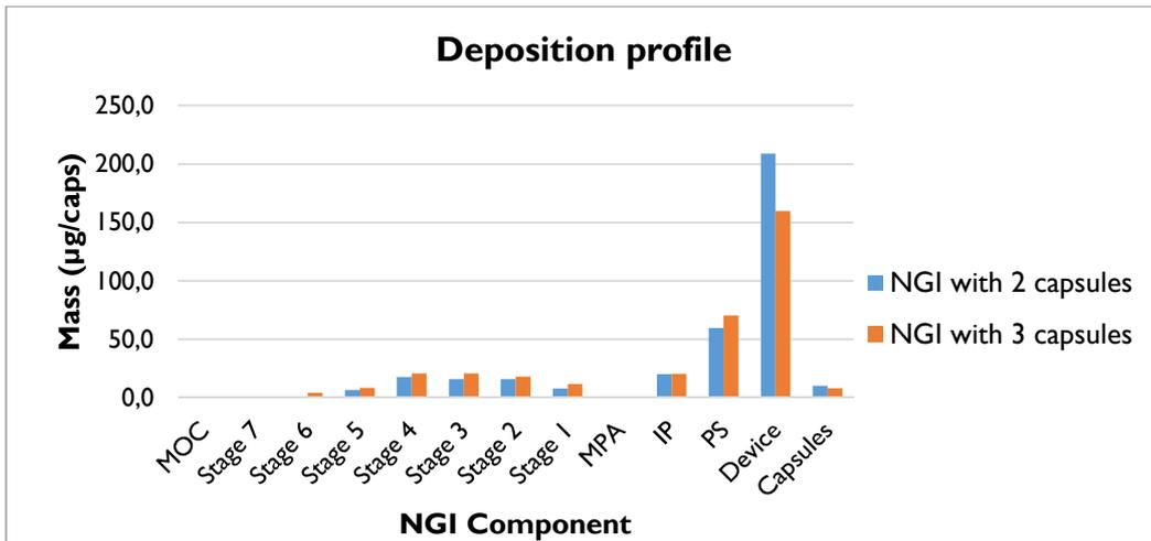
Graphic 3: Comparison between the deposition profile of NGI performed with 2 and 3 capsules.
