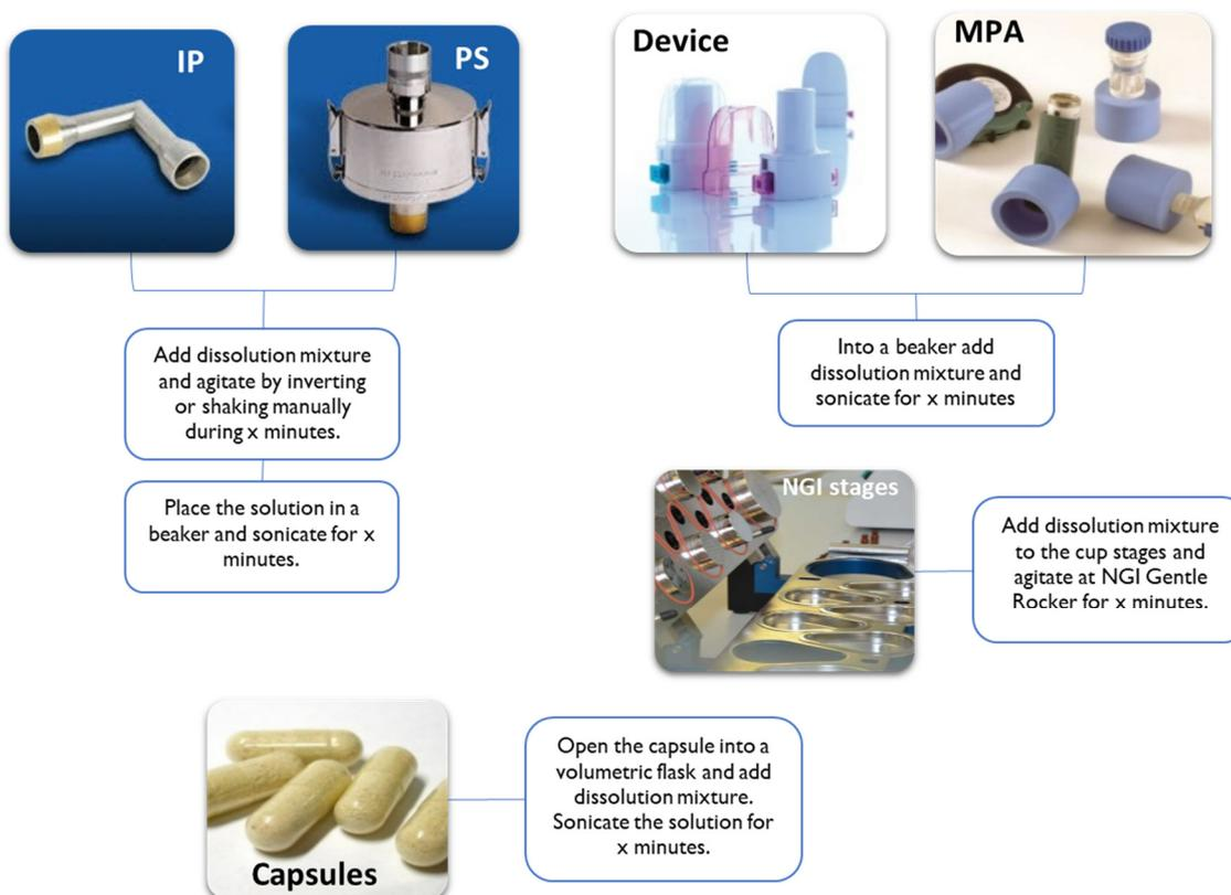
Figure 19: Recovery procedure for API extraction.
