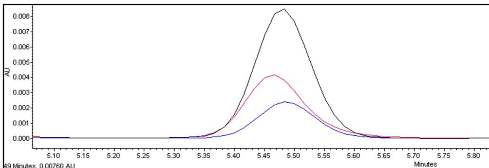
Figure 21: Overlay of the chromatograms obtained by injecting device with API (dark line), device without API sonicated 10 minutes (pink line) and device without API and without sonication (blue line).
