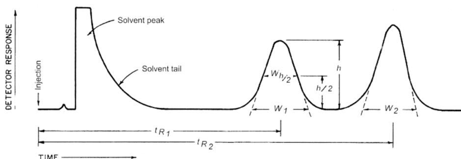
Figure 18: Example of chromatographic separation of two samples (39).
