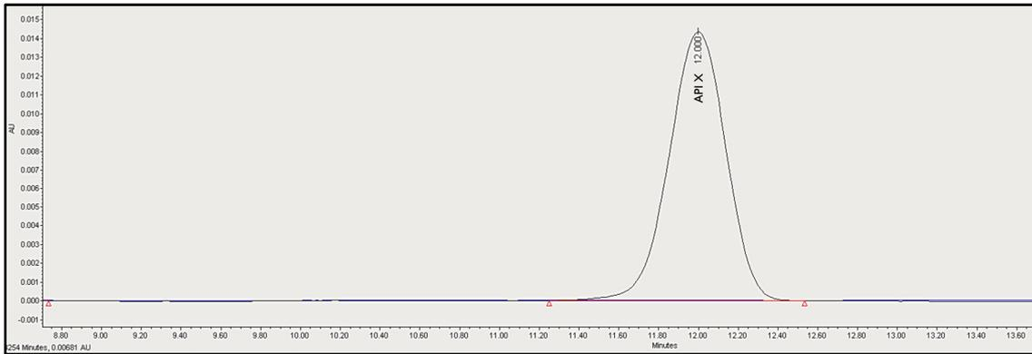
Figure 22: Overlay of chromatogram obtained by injection of device with API (NGI with 10 capsules) and without API (Method II).
