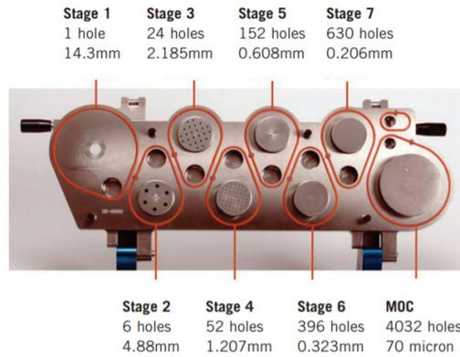
Figure 10: Layout of NGI showing size of nozzles on each stage (30).
