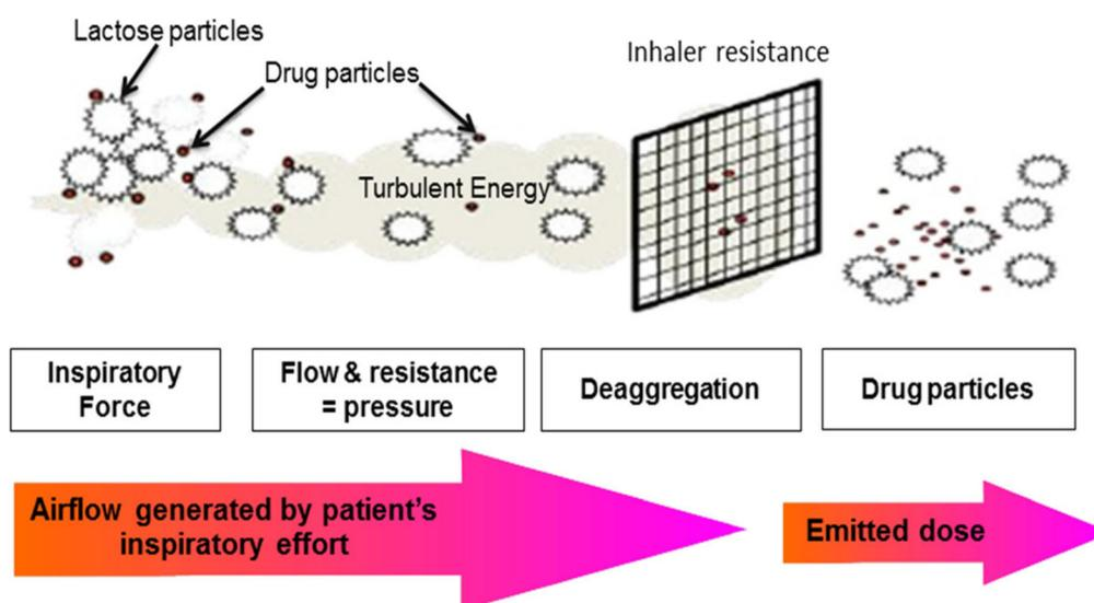
Figure 8: Schematic diagram of carrier-based formulation and dispensing powder mechanisms (14).
