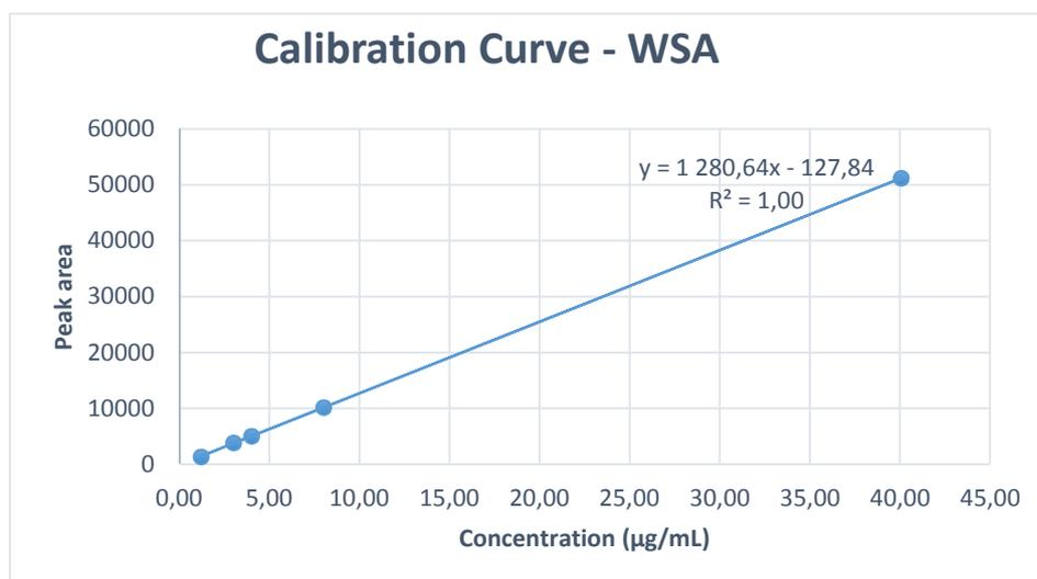
Graphic I: Calibration curve of WSA with equation chart and coefficient of determination ( $r^2$ ).
