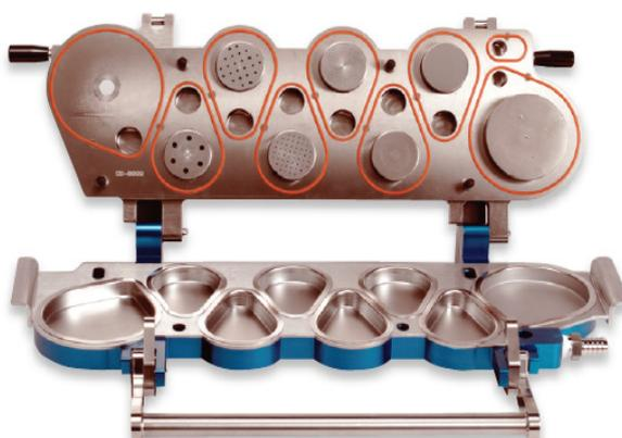
Figure 9: NGI with three main parts. (17)
