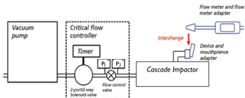
Figure 16: Adaptation of scheme that represents NGI test-setup for DPI testing (34).
