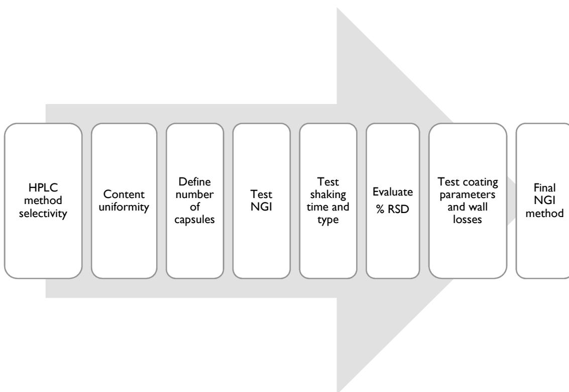
Figure 24: Summary of the fundamental steps necessary to develop a NGI method.
