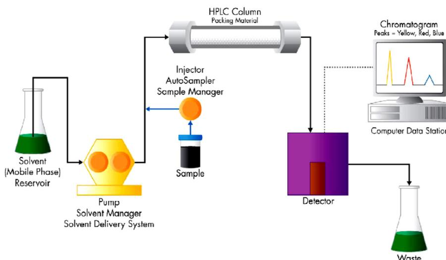
Figure 17: Workflow of an HPLC isocratic system. (37)
