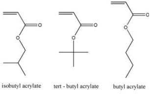
Figure 1. Isomeric structures of butyl acrylate.
