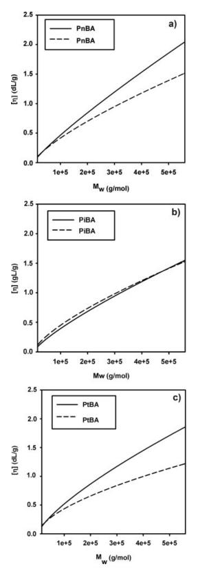
**Figure 5.** Viscosity of PBA isomers prepared by SET and by FRP: (a) PnBA, (b) PiBA, and (c) PtBA (dash line – prepared by FRP; solid line – prepared by LRP).
