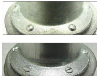
Figure 3.15 – Installation indicators on collar flange before and after installation (Alcoa, 2015), (Fric et al 2014)
