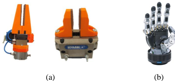
Figure 2- Robotic grippers; (a) Conventional Grippers; (b) Complex robotic gripper Schunk SVH Hand [2].
