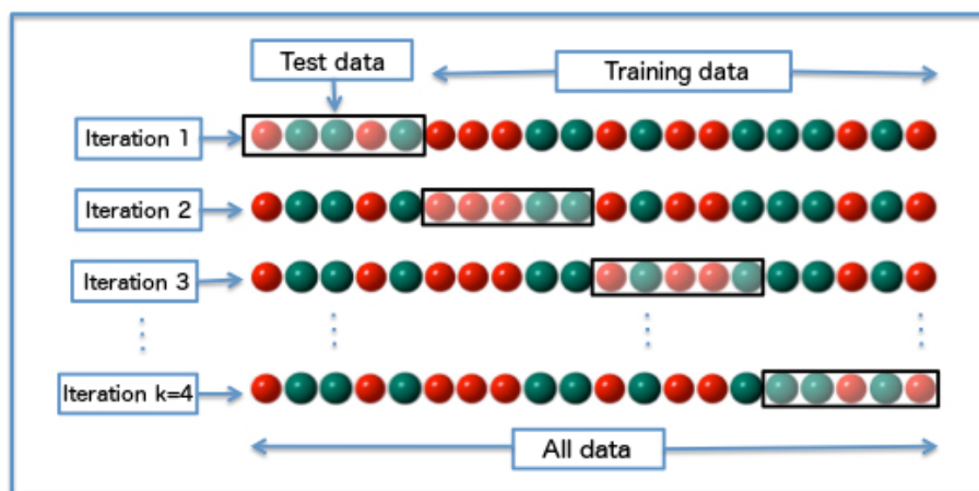
Figure 2.17: Visual representation of a k -fold cross-validation with k = 4 . Image by Fabian Flöck - Own work, CC BY-SA 3.0, https://commons.wikimedia.org/w/index.php?curid=51562781
