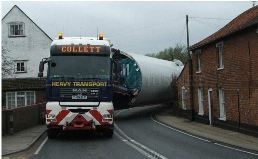
Figure 4.1: Transportation of section of tubular tower ( http://piximus.net/vehicles/transportation-of-the-giant-wind-turbine )
