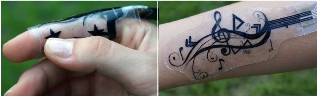
Figure 2.2: iSkin consist on a pattern layer of cPDMS on a PDMS layer [14].
