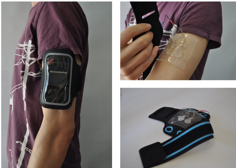
Figure 3.17: The GSR system was placed on the upper-arm of the subject and fixed with an armband.
