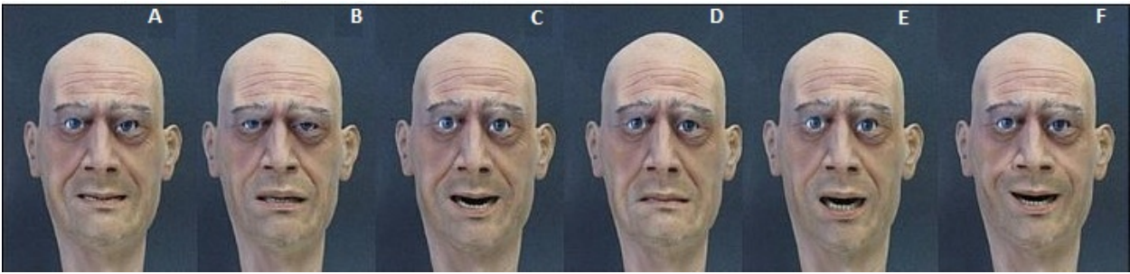
Figure 2.4 Robot ROMAN facial expressions [17]. The expressions' correspondence are as follows: A = anger, B = disgust, C = fear, D = sadness, E = surprise and F = happiness. Taken from [1]
