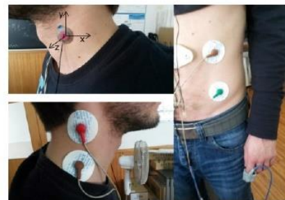
Fig. 1- Top left: location of the accelerometer. Bottom left and right: ECG sensors of the Sensatron. Image adapted from [7].
