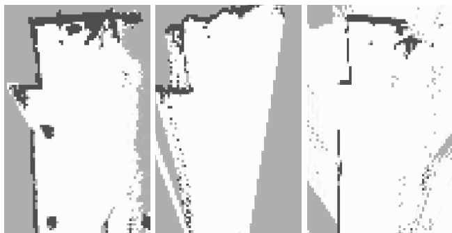
Fig. 5. Results obtained from experiment 2 (from left to right): office traversal with Kinect One using the proposed method, Leddar IS16 using local map and standard ROS package solution using Kinect.
