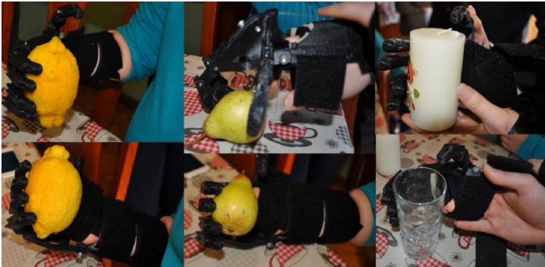
Figure 15 – Testing the cyborg beast prosthesis
