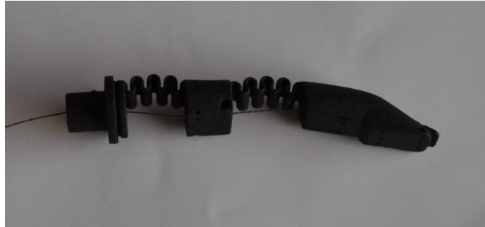
Figure 29 - 3D printed rigid endoskeleton with two joints
