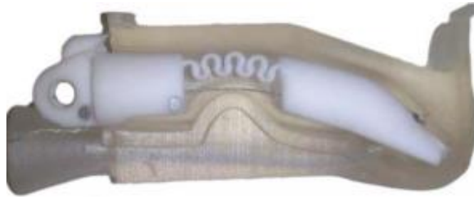
Figure 27 - 3D printed rigid endoskeleton [35]
