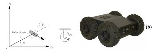
**Figure 2.9.** Kinematics constrains **[3]** and examples of mobile robots using four wheels as locomotion mechanism: a) steered standard wheel, Adept Mobile Robots Seekur system **[21]**, b) fixed standard wheel, Dr. Robot Jaguar 4x4 Mobile Platform **[22]**.
