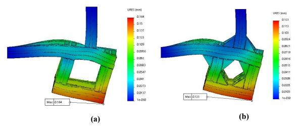
Figure 3.14. Deformation results, top view: a) Without fastenings and b) with fastenings.
