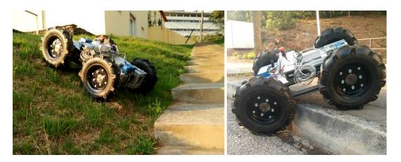
(a) (b) Figure 4.5. Challenging Hunter: a) climbing 30° slope, b) climbing a 200 mm step.
