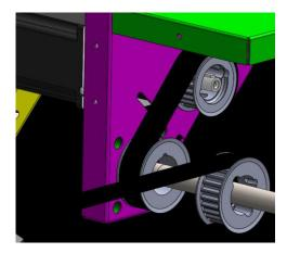
Figure 3.3. Motion transmission between the motor and the wheel using two pulleys and one belt.
