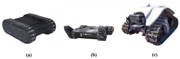
Figure 2.12. Tracked mobile robots: a) Super-Size HD Tracked Tank Robot [27], b) Jaguar V4 Tracked Mobile Robotic Platform [28], c) XBOT All Terrain Tracked Mobile Robot [29].
