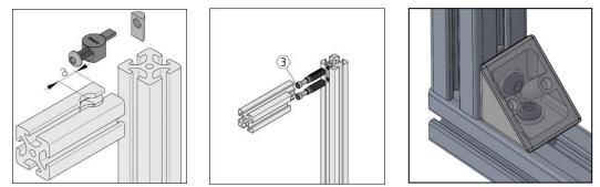
Figure 3.12. Automatic-Fastening, Universal-Fastening, Angle Bracket [38].
