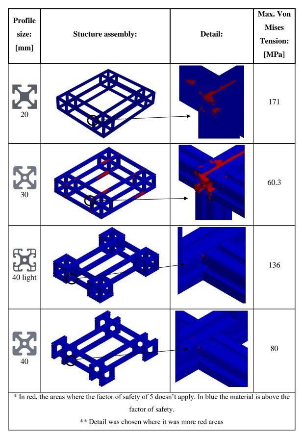
Table 3.6. Factor of safety, Maximum Von Mises tension criterion.
