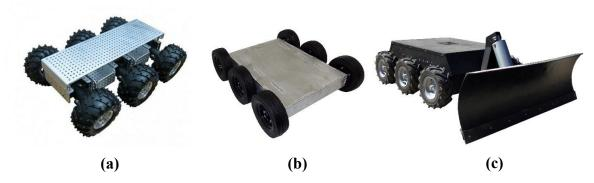
Figure 2.10. Mobile robots with six wheels: a) 6WD Wild Mobile Platform [23], b) Super Droid Robots 6WD All Terrain Robot Platform [24], c) Custom RC 6WD Robot with Snow Plow [25].
