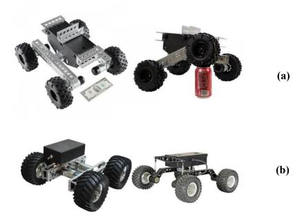
Figure 2.1. Skid Steer robots with flexible structure: a) Nomad 4WD Off-Road Chassis Kit [11], b) Gears EdS-Heavy Metal Articulating Chassis (left) and Gears EdS - Surface Mobility Platform (right) [12].
