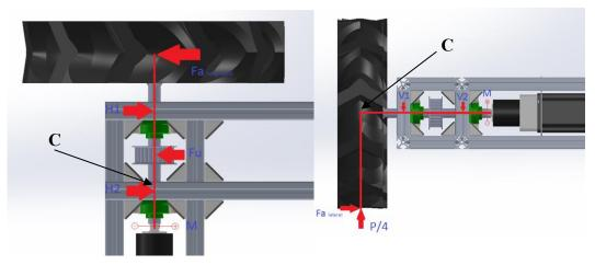
Figure 3.5. On the left: top view (horizontal) of one quarter of the robot, and front view (vertical) on the right, both with forces and momentums applied.
