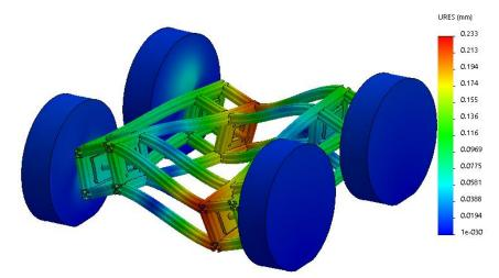
Figure 3.11. Deformation result for the model developed (figure 3.10).
