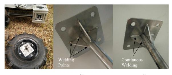
(a) (b) (c) Figure 4.3. First problem, testing in rough conditions: a) Broken wheel, b) Shaft before new welding, c) shaft after new welding.
