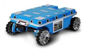
Figure 2.16. Hangfa Navigator Q2 Robot Platform, with four 45 degrees QMA-15 omni wheels [36].
