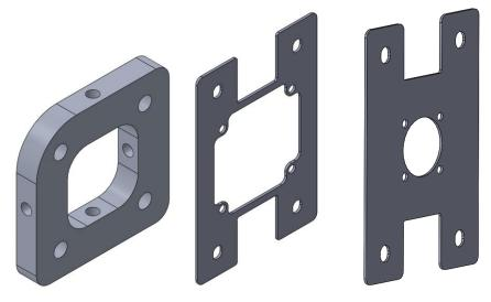
Figure 3.15. Components designed and manufactured, 2D designs in appendices.
