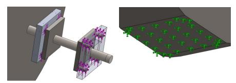
Figure 3.10. Model of the robot, forces in purple and restrictions in green.
