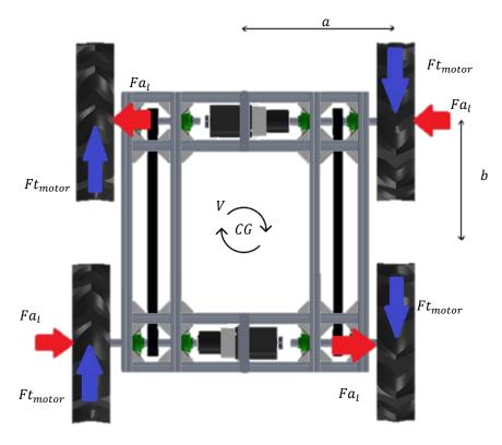
Figure 3.6. Top view of the robot; movement around his geometric centre with forces in each wheel.
