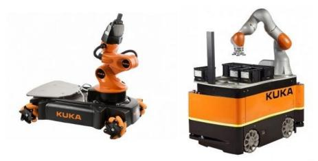
**Figure 2.15.** KUKA youBot **[34]** on the left, mainly used in research and teaching. It consists of an omnidirectional mobile platform on which a five-axis robot arm with a two-finger gripper is installed. On the right KUKA KMR iiwa **[35]**, having the same technology but more prepared for practical applications.
