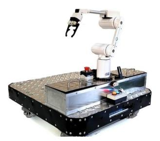
Figure 1.3. Forte, semi-industrial R&D robotic platform [4].
