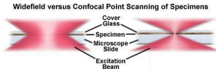
Figure 2.6 - Light focus on widefield conventional microscopy against confocal microscopy. (Microscopy Resource Center)
