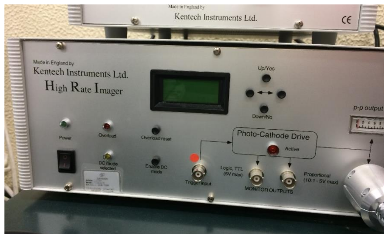
Figure 3.13 - HRI controller Module
