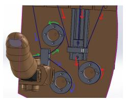
Figure 2.8: Schematic of how the actuators work in ISR-SoftHand
