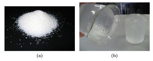
**Figure 2.25:** (a) Sodium polyacryate in its pure state; (b) Hydrogel made by adding water to sodium polyacrylate.
