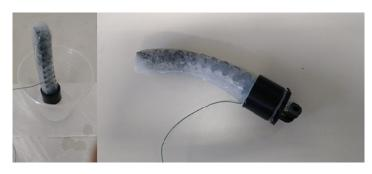
Figure 3.12: Little mold cure and removal of the thin perimeter after curing.
