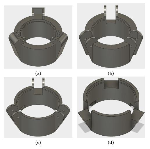
**Figure 4.2:** Grippers body iterations: (a) Initial body; (b) First iteration; (c) Second iteration; (d) Final version.
