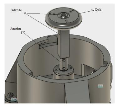
Figure 4.8: Second assemble of the soft gripper.
