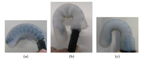
Figure 5.1: Full flexion of the soft finger: (a) Finger fully cured with Ecoflex (22N) was required to make the half flexion); (b) Finger with empty space between the endoskeleton and Ecoflex layer (8N was required to do this flexion, however, the wrinkles on the skin is not optimal for grasping objects, since it reduces the contact area); (c) Finger filled with hydrogel.
