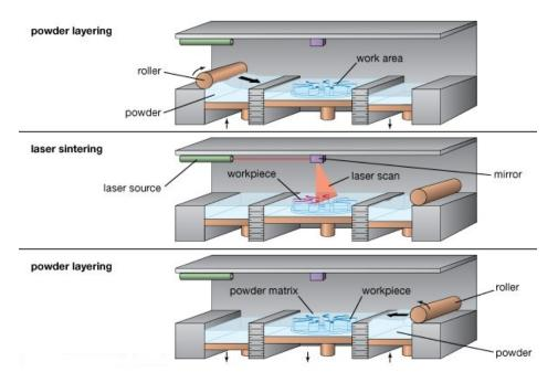
Figure 2.17: Schematic of how SLS printer works [9]
