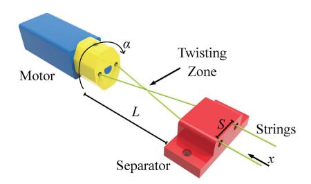
**Figure 2.11:** Twisted string system. With an electric motor (blue), strings (green), connection between motor shaft and strings (yellow) and separator (red). Where L is twisting zone length, a is the rotational angle of the motor shaft, x is the linear displacement of the strings and S is the distance between the holes of the separator.
