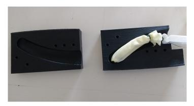
Figure 3.6: Second attempt to create the soft finger by using a latex finger.
