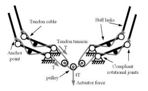
Figure 2.5: Schematic of the SDM Hand
