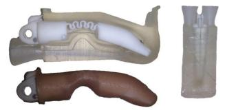
Figure 2- Previous version of the finger with a 3D printed endoskeleton and a soft skin. Due to the buckling effect the skin required to have a curve profile cut on the joints
