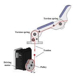
Figure 2.14: Design of the finger and its pulley mechanism made by Song et. Al.
