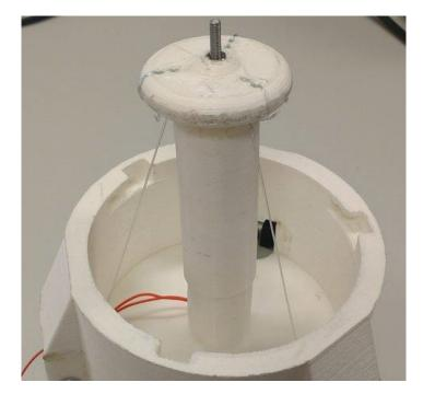
Figure 4.13: Real picture of the final assemble of the soft gripper.
