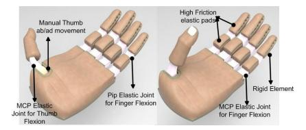
Figure 2.7: Conceptual design of the ISR-Softhand
