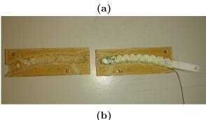
Figure 3.5: First attempt to create the soft finger using flexible polyurethane foam: (a) Endoskeleton finger casted with foam; (b) Endoskeleton finger with foam inside the mold after the curing.
