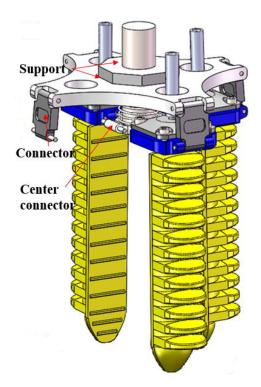
Figure 2.1: Design of the 3D structure of the soft robotic gripper made by Hao et. Al.
