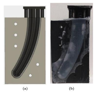
**Figure 3.9:** Longitudinal schematic of both molds: (a) 3D design; (b) Real picture after curing.
