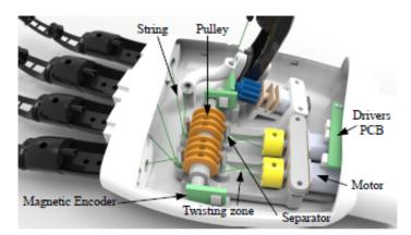
Figure 2.9: 3D model of the UC-softhand
