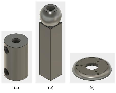
**Figure 4.7:** Gripper pieces: (a) Junction that connects the actuator and the threaded shaft; (b) "BallCube" which is around the threaded shaft; (c) Dish that is attached on the ball which is on top of the "BallCube".
