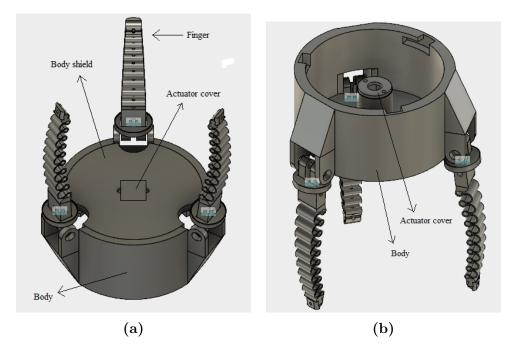
Figure 4.6: First assemble of the soft gripper: (a) Top view; (b) Bottom view.
