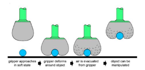
Figure 2.15: Schematic of operation of an universal gripper based on air
