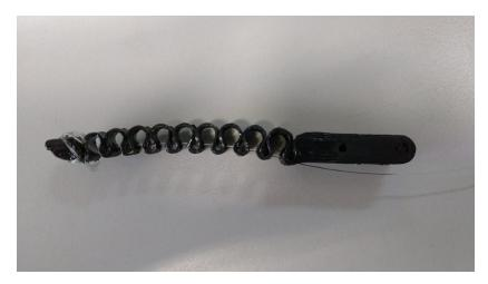
Figure 3.4: 3D printed endoskeleton embebed in acetone
