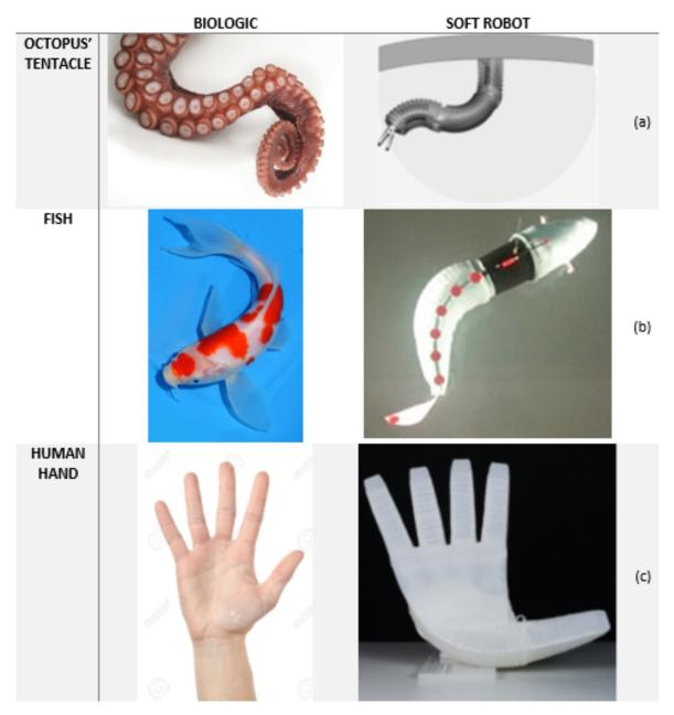
**Table 1.1:** Table that shows similiraties between a biologic organ and a soft robot: (a) Soft robot that resembles an octopus' tentacle used by Cianchetti et al. [14] (b) Soft robot that resembles a fish used by Marchese et al. [15] (c) Soft robot that resembles the human hand used by Deimal et al. [16]
