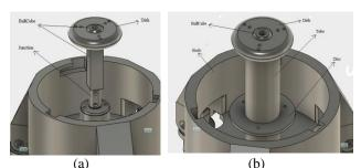
Figure 11- Bottom view of the 3D design of the under actuated gripper: (a) second assemble, (b) third assemble
