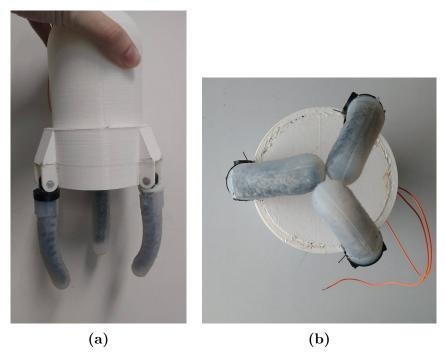
Figure 5.2: Pictures of the under-actuated gripper with the soft fingers integrated: (a) Side view; (b) Top view.
