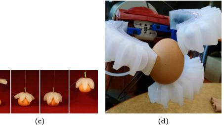
**Figure 1.2:** Examples of soft grippers: (a)Versaball made by Empire Robotics based on the jamming of granular material [6]. (b) Soft Robot made by SoftRobotInc. (c) Ilievski et al. [7]. (d)Homberg et al. [8].
