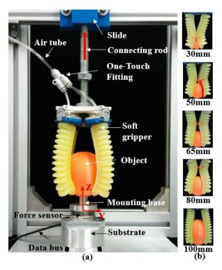
**Figure 2.2:** Apparatus for measuring force of the soft gripper under different effective lengths made by Hao et. Al.. (a) Schematic illustration of the force measurement platform. (b) Images of the soft robotic gripper under five selected effective finger lengths while gripping, regulated with an inelastic nylon tendon.
