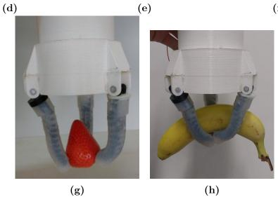
Figure 5.3: Pictures of some grasping tests made with the soft gripper: (a) Apple with 151.92 g; (b) Orange with 140.24 g; (c) Peach with 147.56 g; (d) Duct tape with 66.52 g; (e) Flask with 126.26 g; (f) Ball with 12.46 g; (g) Strawberry with 52.38 g; (h) Banana with 201 g.
