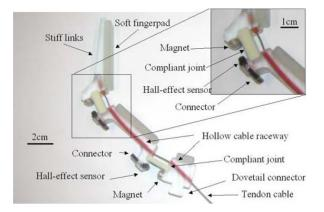
Figure 2.4: Details of the finger parts of the SDM Hand
