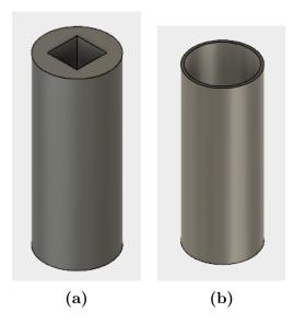
Figure 4.9: Gripper Tube: (a) Squared part of the tube; (b) Circular part of the tube.
