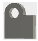
Figure 4.3: Support to attach soft fingers in the gripper body.
