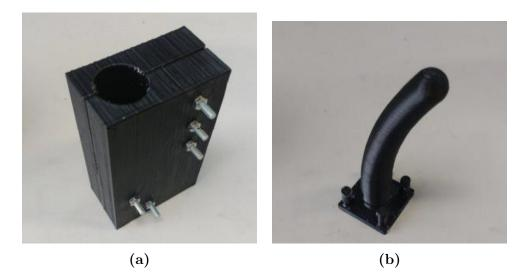
Figure 3.8: 3D printed molds for the Ecoflex curing: (a) Main mold; (b) Shaping mold.
