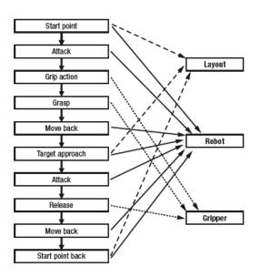
Figure 2.12: Flow chart process of a pick and place operation made by Blanes et. Al.
