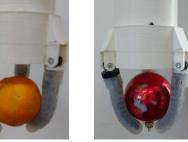
Figure 12- Grasping tests with some objects: (a) Peach with 147,56g; (b) Apple with 151,92g; (c) Ink flask with 126,26g; (d) Cube with 35,62g; (e) Orange with 140,24g; (f) Ball with 14,46g.
