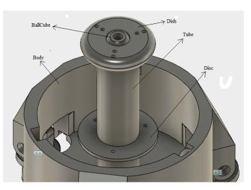
Figure 4.11: Final assemble of the soft gripper.
