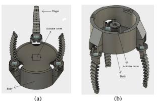
*Figure 10- 3d design of the first assemble of the under actuated gripper: (a) Top view; (b) Bottom view*
