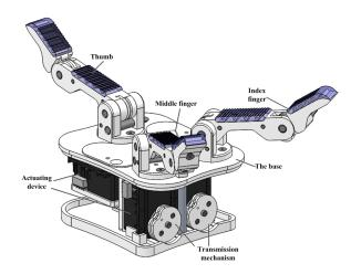
Figure 2.13: Design of the gripper made by Song et. Al.
