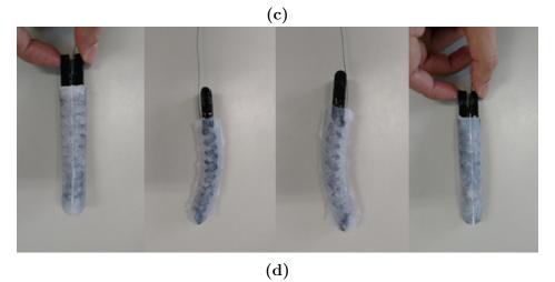
**Figure 3.7:** Failed soft fingers after the hydrogel mixed with Ecoflex cure: (a) Cure attempt with little Ecoflex, (b) Cure attempt with too much hydrogel, (c) Cure attempt with good ratio but not well distributed, (d) Cure attempt with the perfect ratio but with a lot of holes and ecoflex between the joints.
