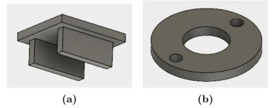
**Figure 4.5:** Actuator covers: (a)Actuator cover attached on top part of the base shield; (b) Actuator cover attached on the bottom part of the base shield.
