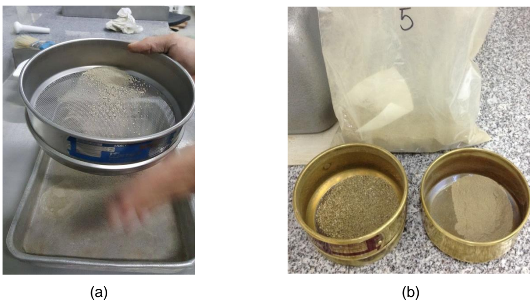
Figure 43 - (a) Sieving process using 1mm Retsch test sieve (b) Sieving process using 0.125mm Endecotts test sieve.
