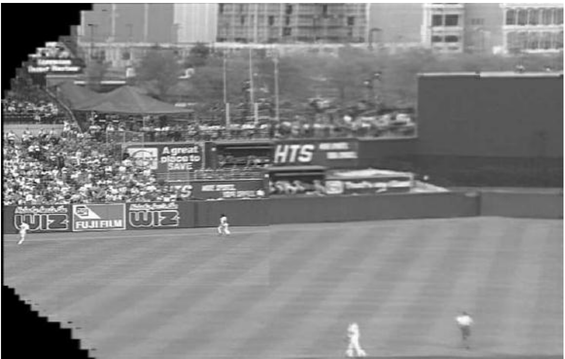
Figure 15. . Static and dynamic mosaicking taken from [48]. Top: Construction of the static mosaic using the temporal median of a baseball game sequence. Bottom: Construction of a dynamic mosaic of a baseball sequence.
