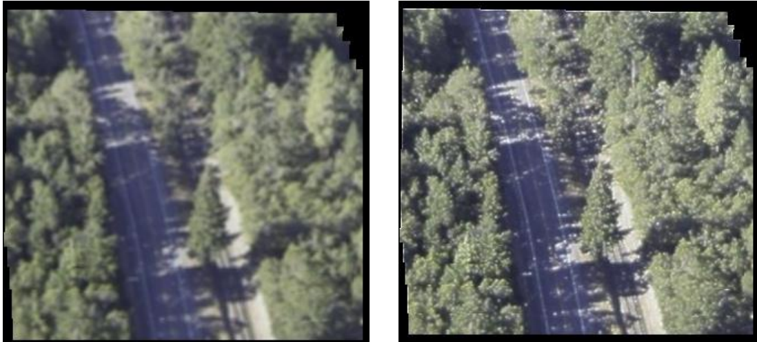
Figure 46. Results of super-resolution mosaicking using the steepest descent algorithm. Left: LR mosaic. Right: the SR mosaic. The mosaic was constructed using five frames of size 320x240x3 pixels.
