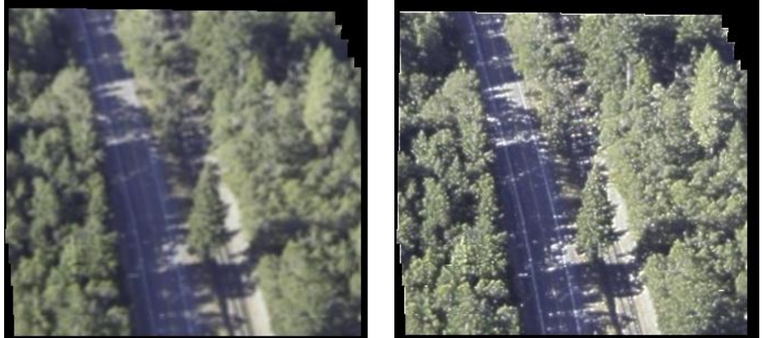
Figure 52. Results of super-resolution mosaicking using the conjugate gradient algorithm. Left: LR mosaicking. Right: SR mosaic. The mosaics were constructed using five frames of a size of 320x240x3 pixels.
