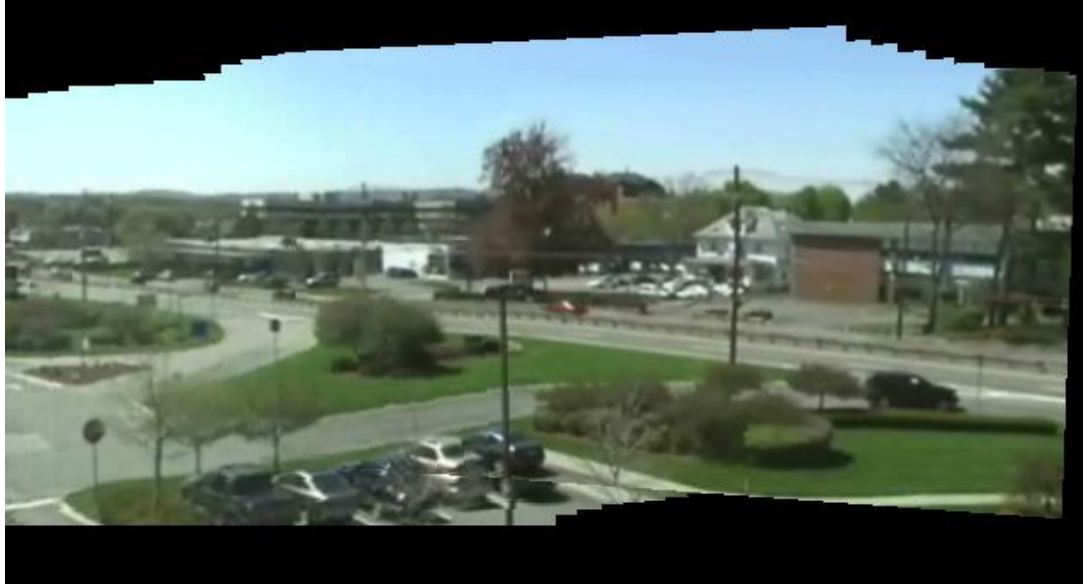
Figure 36. Video mosaicking for 4 seconds at 15 frames per second taken from the video mosaicking demonstration in MATLAB/Simulink.
