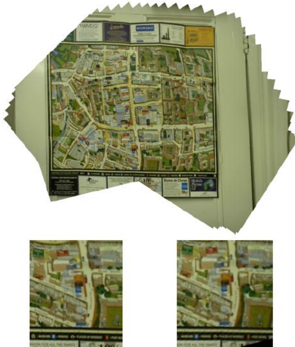
Figure 21. Top: A mosaic image after refinement of the homography by bundle-adjustment, obtained from [31]. Left: A close-up view of the region of interest (red box of the Figure 20). Right: The corresponding region extracted from a single frame.
