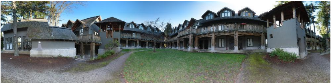
Figure 18. Final mosaic taken from [55]. This mosaic was constructed using 80 images matched using SIFT (Scale Invariant Feature Transform), rendered in spherical coordinates, and blended using the multi-band technique.
