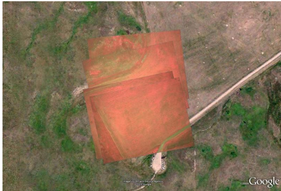
Figure 41. Example of geo-referenced images using images from a color (red, green) and near infrared (false color composite) camera along with GPS and IMU information. (Photo: Courtesy of David Dvorak) .
