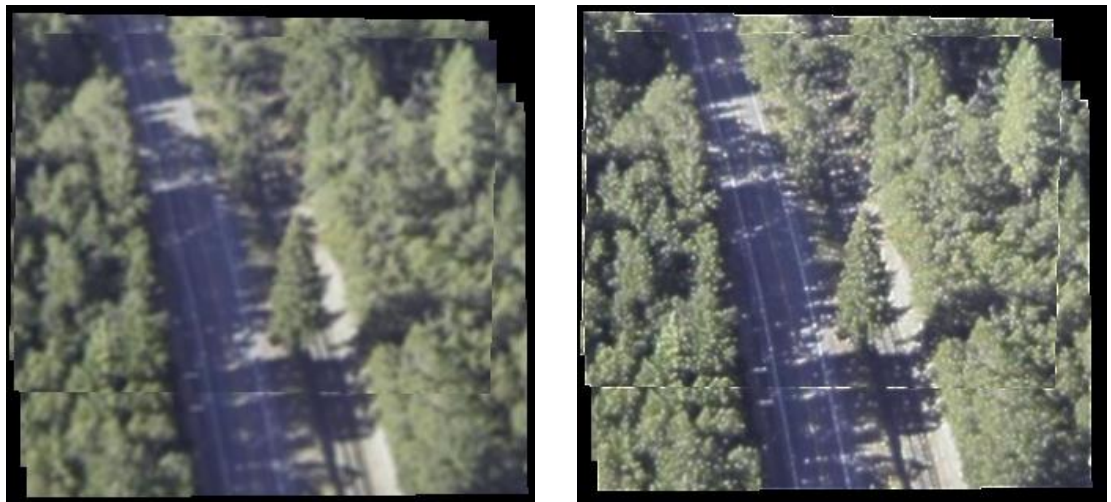
Figure 67. Result of super-resolution mosaicking using steepest descent implemented over GPU-CPU. Left: LR mosaic. Right: SR mosaic. The mosaics were constructed using five frames of size 320x240x3 pixels.
