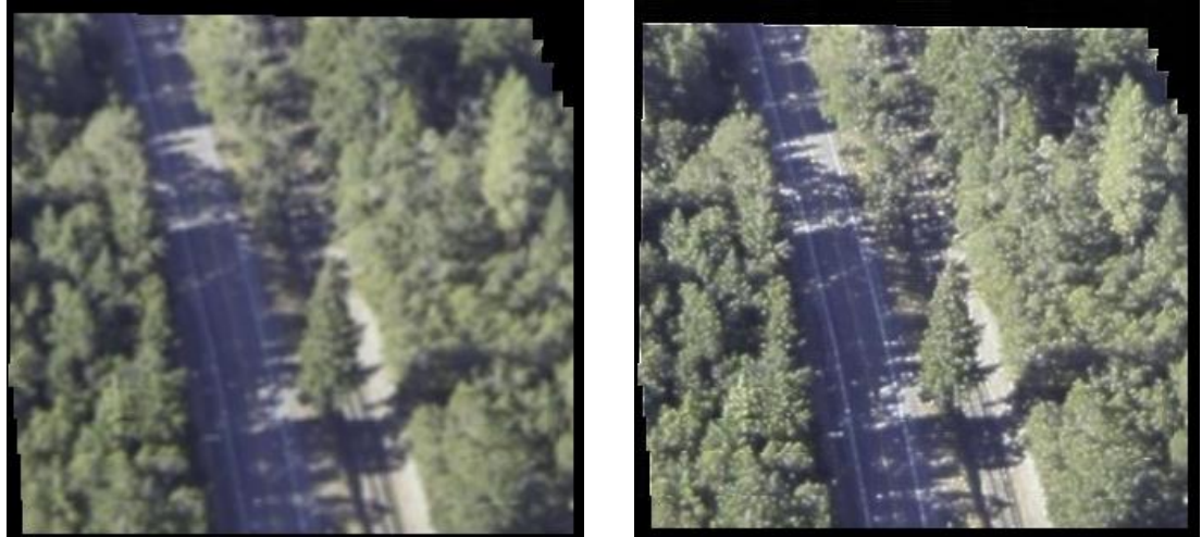
Figure 55. Result of super-resolution mosaicking using the proposed Levenberg Marquardt method. Left: LR mosaicking. Right: SR mosaicking. The mosaics were constructed using five frames of size of 320 \times 240 \times 3 pixels.
