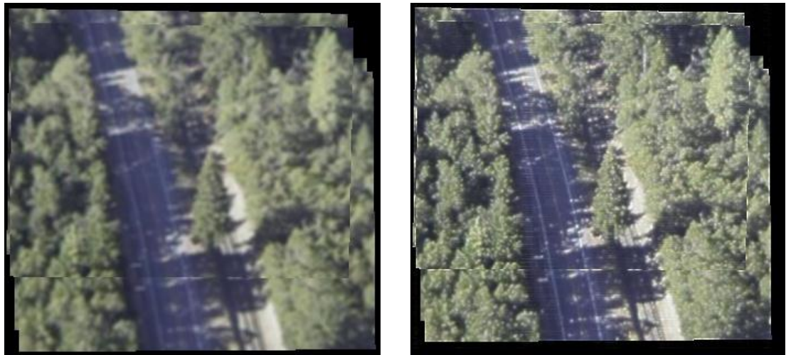
Figure 73. Results of super-resolution mosaicking using the Levenberg Marquardt algorithm implemented over GPU-CPU. Left: LR mosaic. Right: SR mosaic. The mosaics were constructed using five frames of size 320x240x3 pixels.
