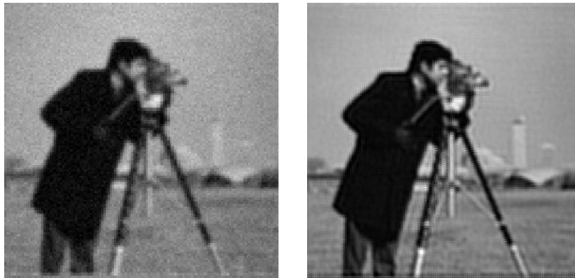
Figure 5. Example of frequency-domain approach for super-resolution taken from Tom and Katsaggelos [20, 21]. Left: One of the four synthetic LR images. Right: SR image. There are several ringing artifacts, particularly along the image edges, but there is also a distinct improvement in the resolution of the image.
