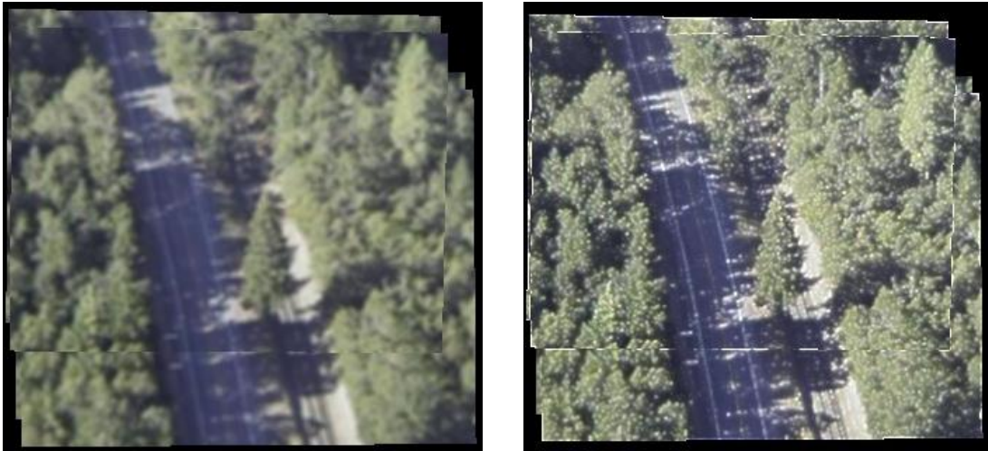
Figure 70. Results of super-resolution mosaicking using the conjugate gradient algorithm implemented over GPU-CPU. Left: LR mosaic. Right: SR mosaic. The mosaics was constructed using five frames of size 320x240x3 pixels.
