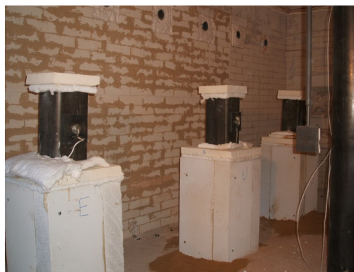
Figure 4.3. Location of test specimens in furnace [97]
