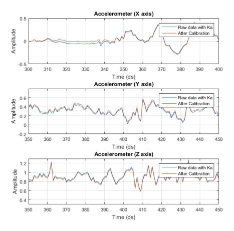
The following figure represents an example of calibration with the available sensor board, for comparison purposes the scale factor  $K_a$  was included with the raw data.
