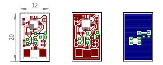
Fig. B.4 Finger board PCB design.
