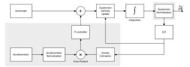
Fig. 2.9 Explicit complementary filter block diagram.
