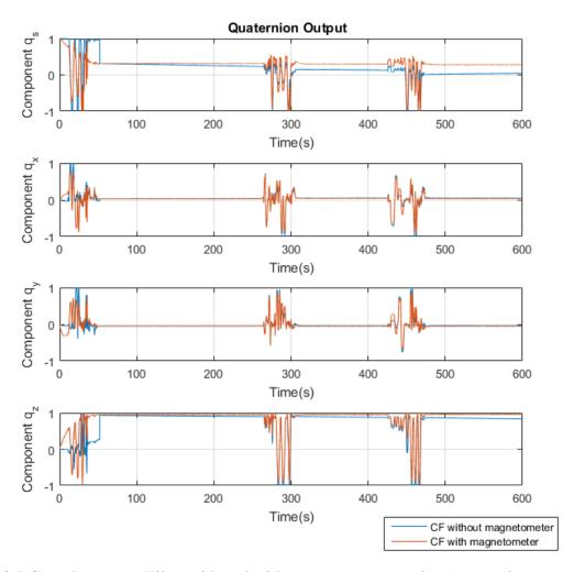
Fig. 3.7 Complementary Filter with and without magnetometer data (quaternion representation).
