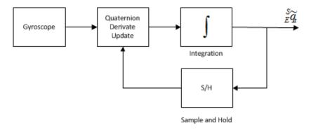
Fig. 2.8 INS orientation estimation block diagram.
