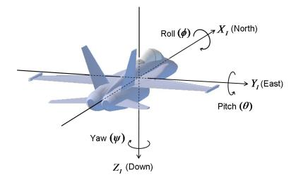
Fig. A.1 Euler angles as described in aeronautical conventional.
