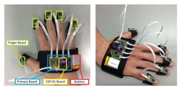
Fig. 4.6 Hand-Tracker prototype.
