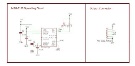
Fig. B.3 Finger board schematic diagram.
