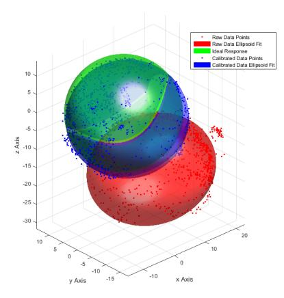
Fig. 2.6 Magnetometer calibration example.
