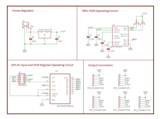
Fig. B.1 Primary board schematic diagram.
