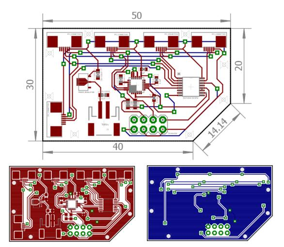
Fig. B.2 Primary board PCB design.
