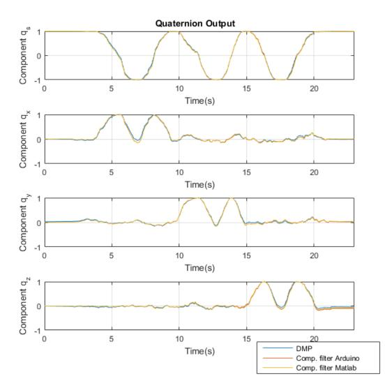
Fig. 3.4 Complementary filter algorithm vs. DMP output.
