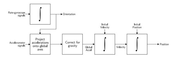
Fig. 2.7 Strapdown Inertial Navigation algorithm.
