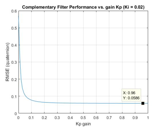
Fig. 3.10 Performance of Complementary Filter as function of  $K_p$ .
