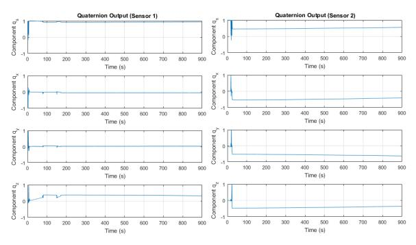
Fig. 3.5 Complementary filter stationary drift (quaternion representation).
