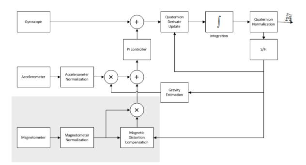
Fig. 2.10 Complementary filter with magnetometer block diagram.
