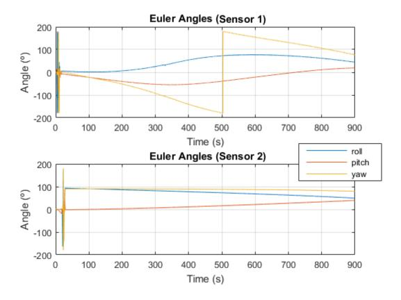
Fig. 3.3 INS algorithm stationary drift (Euler angles representation).
