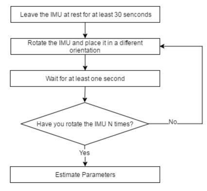
Fig. 2.4 Calibration protocol flowchart.
