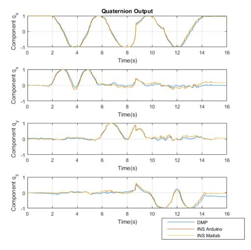
Fig. 3.1 Standard INS algorithm vs. DMP output.
