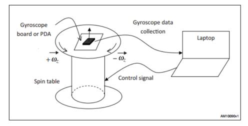
Fig. 2.2 Gyroscope calibration setup.
