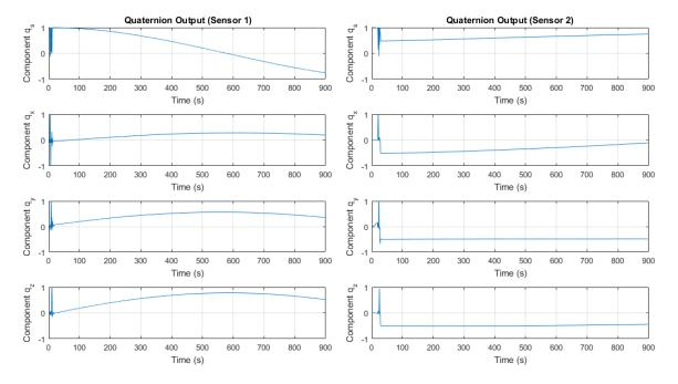
Fig. 3.2 INS algorithm stationary drift (quaternion representation).
