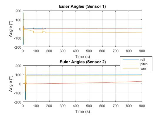
Fig. 3.6 Complementary filter stationary drift (Euler angles representation).
