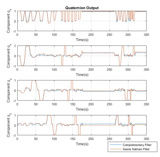
Fig. 3.9 Complementary Filter vs. Xsens Kalman Filter.
