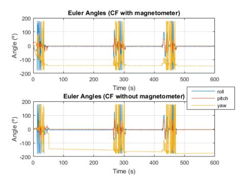
Fig. 3.8 Complementary Filter with and without magnetometer data (Euler angles representation).
