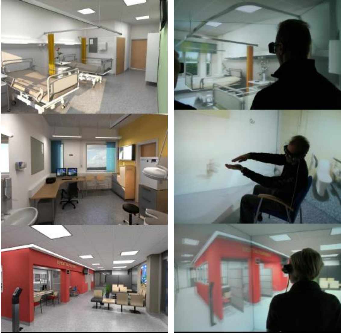
Figure 24 - A collective visualization in CAVE about the design of the Hospital District of South Ostrobothnia , image released by Uki Arkkitehdit
