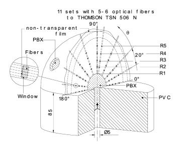
Figure 1. Experimental setup to characterize the shape and detonation velocity of the divergent detonation wave.
