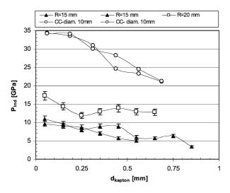
**Figure 8.** Pressure induced on barrier by a divergent DW and by a positive curvature DW (CC-cylindrical charge).
