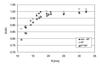
**Figure 4.** Velocities of the divergent detonation wave as a function of the radial distance for different  $\theta$  angles.
