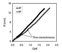
**Figure 5.** Non-monotonous (pulsing) development of the divergent DF in PBX based on RDX registered under two directions of propagation [10]:  $45^{\circ}$  and  $90^{\circ}$ .
