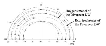
**Figure 3.** Experimental isochrones of the divergent DF (solid lines) and isochrones obtained with the Huygens model (dashed lines).
