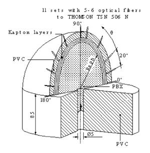
**Figure 6.** Experimental setup to measure the induced pressure in an inert barrier.
