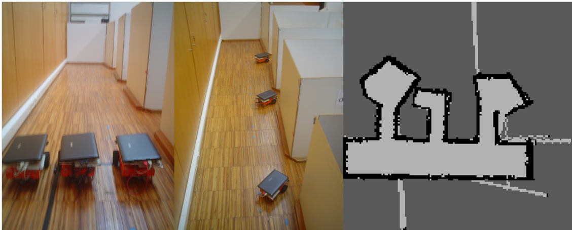
Figure 5.8: Experiment with real robots running the Rapyuta-adapted mrgs system.
