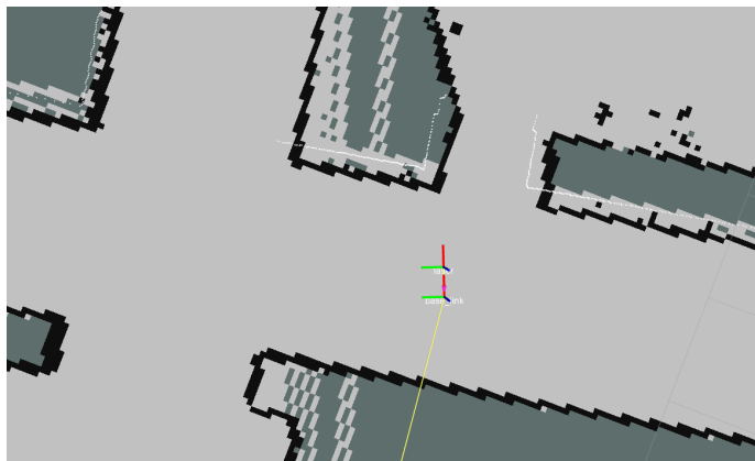
Figure 6.6: Rviz representation of a situation where the localization using AMCL fails.
