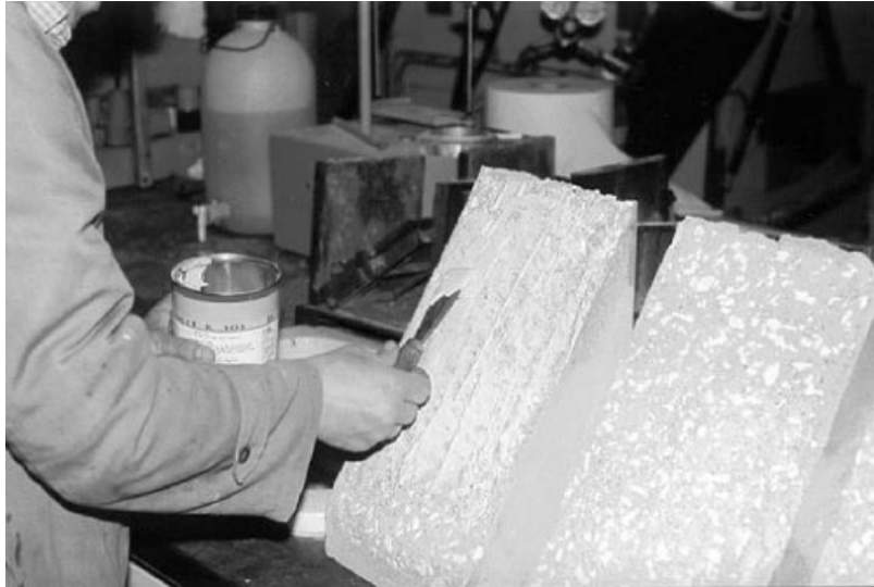
Fig. 4 Epoxy resin application on slant shear specimens prepared by sand-blasting
