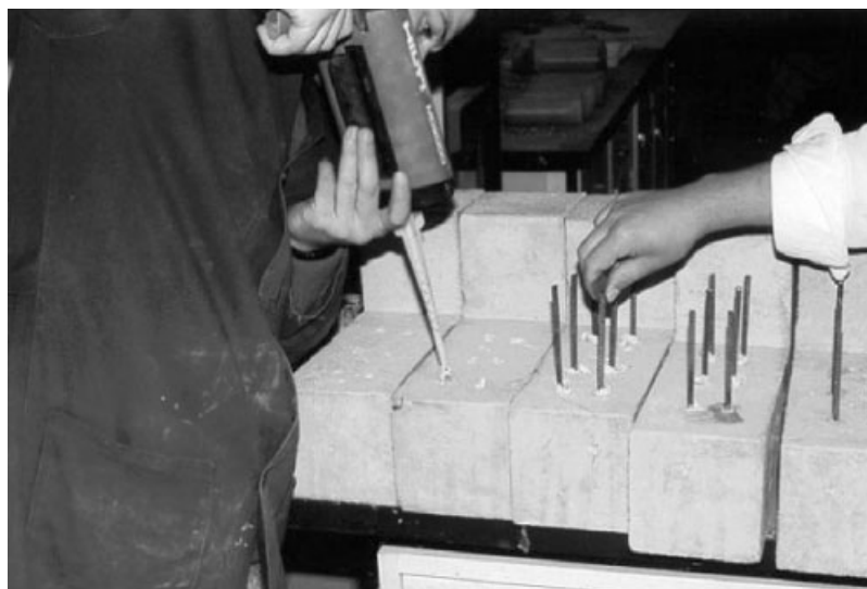
Fig. 5 Steel connectors epoxy bonded on push-off specimens
