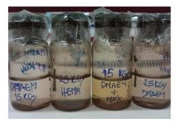
Figure 2-2 - Vials with the membranes after irradiation.
