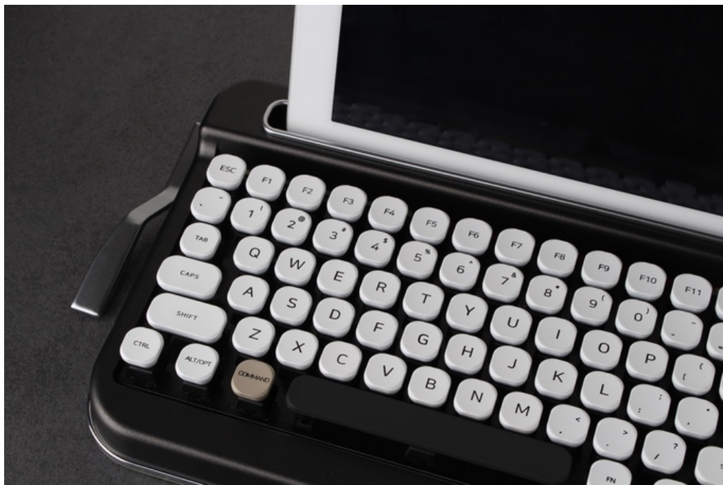
Fig. 3.18: “PENNA,” a bluetooth wireless retro keyboard for iPad that emulates a typewriter’s keyboard. Source: < https://www.theverge.com/circuitbreaker/2017/4/7/15221566/penna-retro-typewriter-bluetooth-keyboard-kickstarter >, last accessed July, 30 2017.
