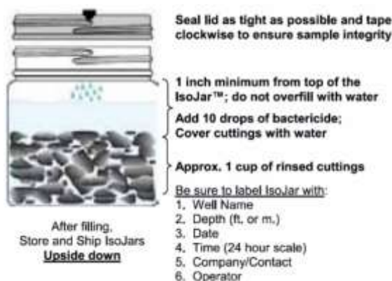
Figure 4.9: An example of the label on the Isojar—complete the label with all information available. Adapted from Isotech (2014).
