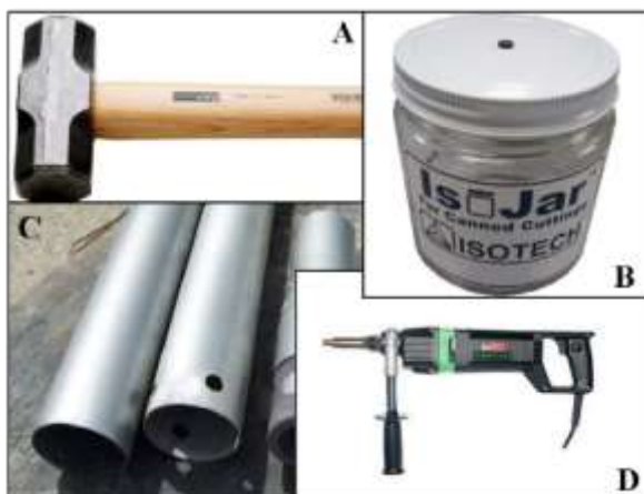
Figure 4.3: A) Hammer; B) Isojar, by Isotech (Weatherford); C) Tubes used for soil sampling; D) Drilling machine used for deeper sampling.
