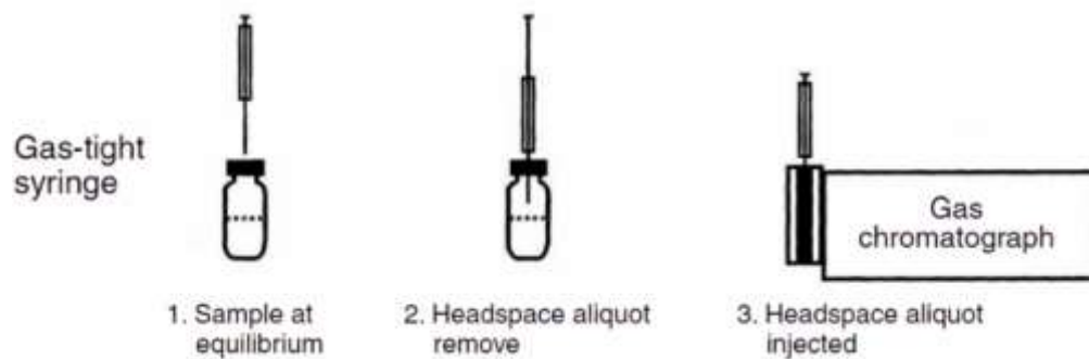
Figure 4.10: The designs of static headspace injection systems used for the analyzes. The gas-tight syringe system uses a syringe to collect and transfer a headspace aliquot to the GC. Adapted from B'Hymer (2010).
