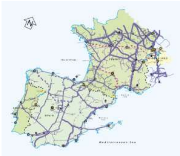
Map 8.1: The European natural gas network (Portugal, Spain, France and Switzerland) – Capacities at cross-border points on the primary market. The pipelines are represented by grey lines. Adapted from European Network of Transmission System Operators for Gas (2016).
