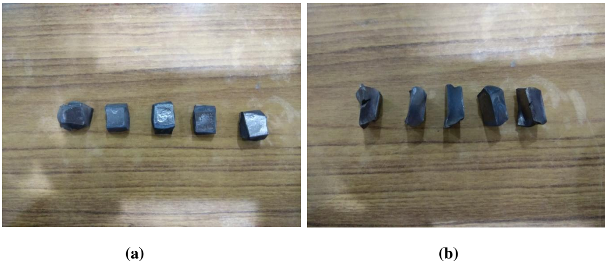
Fig. 51: (a), (b) shows the samples after hot compression
