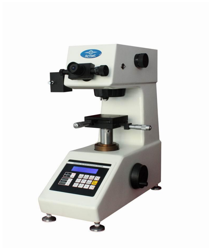
Fig. 21: Micro Vickers hardness tester
