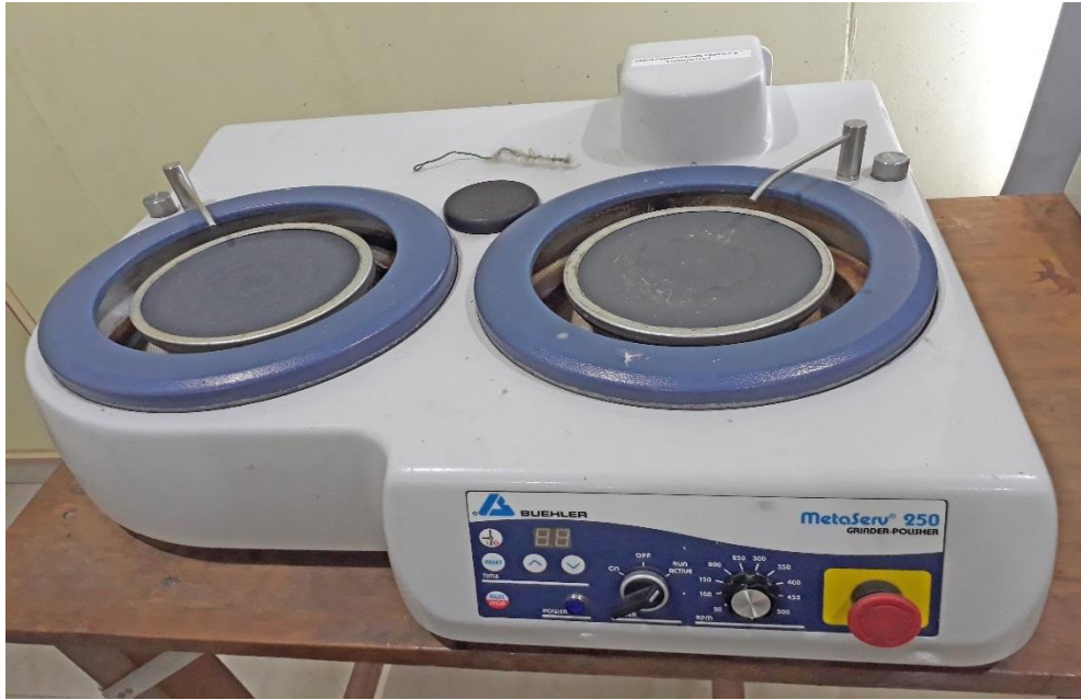
Fig. 16: Double disc polishing machine
