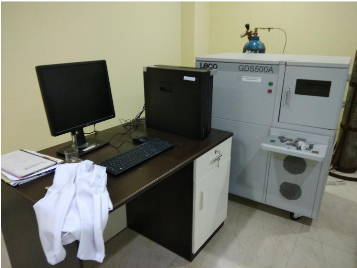
Fig. 9: OES(Optical Emission Spectroscopy)
