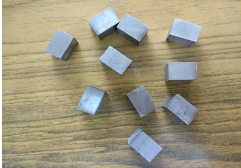
Fig. 50: Samples prepared for hot compression in Gleeble 3800
