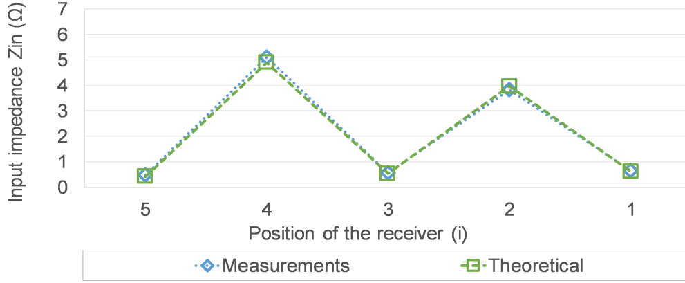
Figure 2.28: Comparison of \hat{Z}_{in} ( \Omega ) measured with the VNA to that calculated through (2.70) using (2.49) for different positions of the receiver, at the resonant frequency f_0 = 147 kHz.
