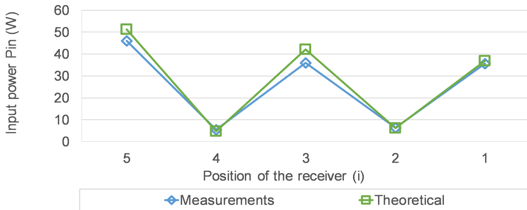
Figure 2.30: Comparison of P_{in} (W) at the resonant frequency f_0 = 147 kHz obtained with measurements using (2.72) to the one calculated through developed formulas ((2.71) using V_s = 4.9V determined with (2.73) and (2.49)) for different positions of the receiver ( i ).
