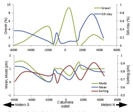
Fig. 7. Pattern of variation of grain-size parameters in beach sediments near the Catumbela outlet.
