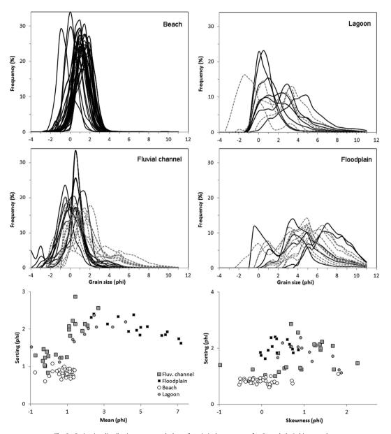
Fig. 3. Grain-size distribution curves and plots of statistical parameters for Catumbela-Lobito samples.
