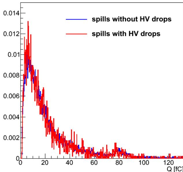
**Figure 11.** Cluster charge distributions recorded in the *Double3* THGEM+SRWELL detector (of figure 10) with pions at a rate of  $3 \frac{\text{kHz}}{\text{cm}^2}$ . The distributions were measured during spills with (red) and without (blue) micro-discharges in the same operation conditions:  $\Delta V_{\text{SRWELL}} = 550 \text{ V}$ ,  $\Delta V_{\text{THGEM}} = 550 \text{ V}$  and  $\Delta V_{\text{Transfer}} = 50 \text{ V}$  resulting in an effective gain of  $\sim 2500$ .
