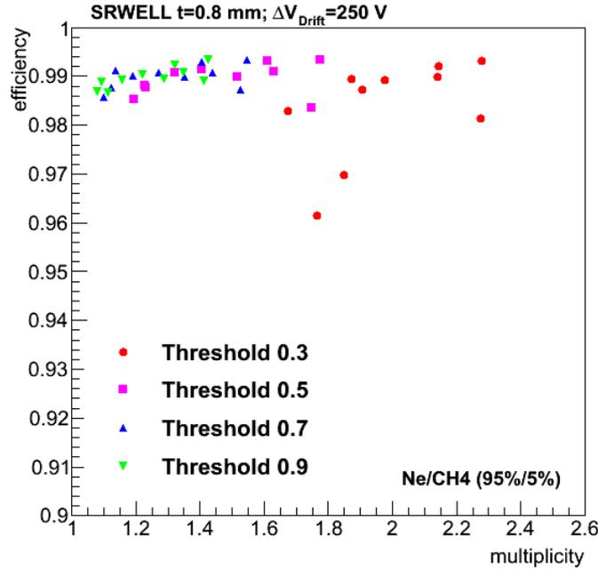
**Figure 4.** Global detection efficiency as a function of the pad-multiplicity for different charge thresholds set in the analysis, as measured with a 0.8 thick SRWELL (figure 2a) with muons. Ne/5%CH<sub>4</sub>;  $\Delta V_{\text{Drift}} = 250$  V.
