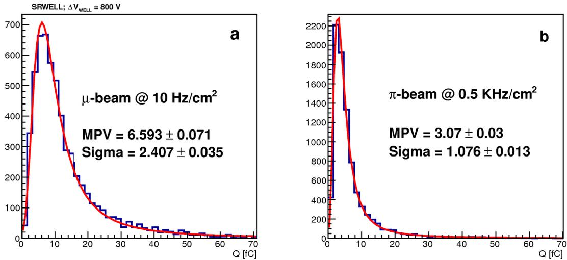
**Figure 8.** Cluster charge distributions measured with the Single2 configuration (table 1) at an operation voltage  $\Delta V_{\text{SRWELL}} = 800 \text{ V}$  (a) muons,  $10\text{--}20 \frac{\text{Hz}}{\text{cm}^2}$ ; (b) pions,  $0.5 \frac{\text{kHz}}{\text{cm}^2}$ . The measured data (blue histograms) are fitted to Landau distributions.
