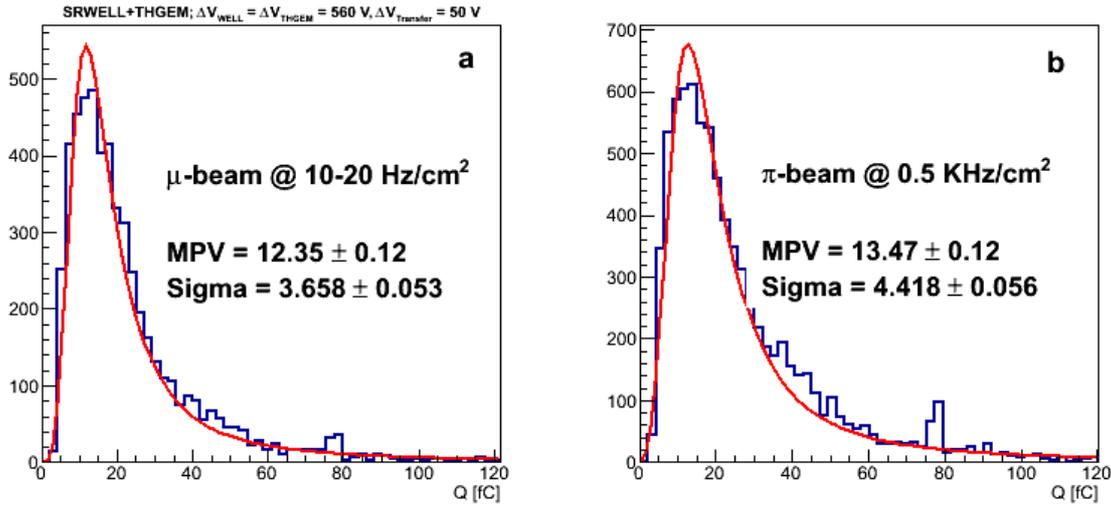
**Figure 9.** Cluster charge distributions measured with the *Double1* configuration (table 1) at operation voltages  $\Delta V_{\text{SRWELL}} = 560 \text{ V}$ ,  $\Delta V_{\text{THGEM}} = 560 \text{ V}$  and  $\Delta V_{\text{Transfer}} = 50 \text{ V}$ . (a) Muons, 10–20  $\frac{\text{Hz}}{\text{cm}^2}$ ; (b) pions, 0.5  $\frac{\text{KHz}}{\text{cm}^2}$ . The measured data (blue histograms) are fitted to Landau distributions.
