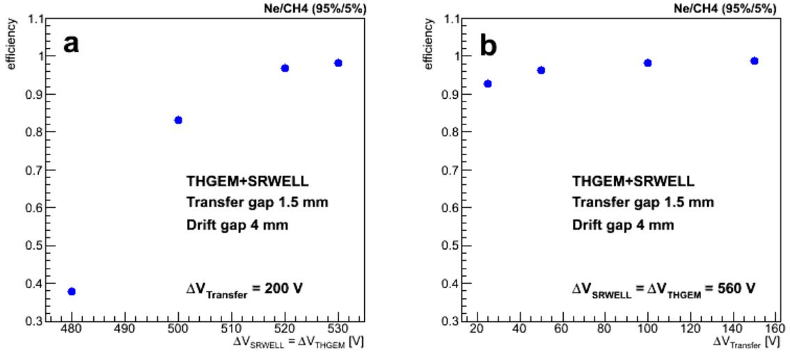
**Figure 5.** The detection efficiency with muons of the THGEM+SRWELL in a *Double1* configuration (figure 2b; table 1) as a function of applied potential. (a) Efficiency as a function of the voltage across both multipliers ( $\Delta V_{SRWELL} = \Delta V_{THGEM}$ ) at constant  $\Delta V_{Transfer} = 200$  V; (b) efficiency as a function of the  $\Delta V_{Transfer}$  at constant  $\Delta V_{SRWELL} = \Delta V_{THGEM} = 560$  V.
