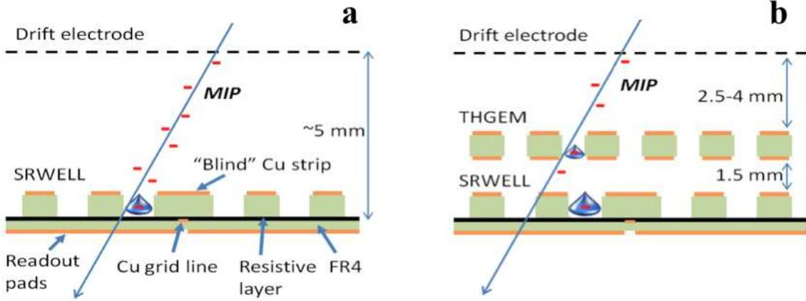
**Figure 2.** Schematic views of the SRWELL detector (a) and the double-stage THGEM+SRWELL (b) configurations. Avalanche charges induce signals through a resistive anode, onto pads located behind a  $100\ \mu\text{m}$  thick insulator. The copper-grid below the resistive film evacuates the electrons diffusing across its surface.
