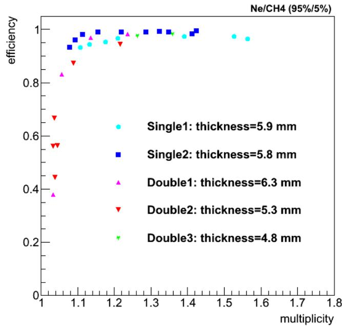
**Figure 6.** Detection efficiency with muons as a function of the pad multiplicity measured with the single-SRWELL and the double THGEM+SRWELL configurations listed in table 1. The total detector thickness, excluding readout electronics, is provided for each case in the figure. The optimal voltages and resulting efficiency, multiplicity and gain values are given in table 2.
