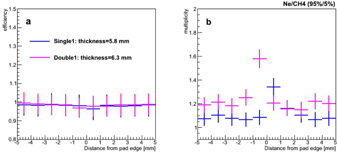
**Figure 7.** Local efficiency and multiplicity data measured with the Single2 SRWELL and the Double1 THGEM+SRWELL, using the tracking system. (a) Detection efficiency as a function of distance from the edge of the pad. (b) Pad multiplicity as a function of distance from the edge of the pad. The operation potentials are depicted in table 2.
