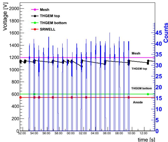
**Figure 10.** The *Double3* THGEM+SRWELL detector configuration. High-voltage variation in time overlaid on the spill structure, as measured in a pion beam at a rate of  $3 \frac{\text{kHz}}{\text{cm}^2}$ . No high voltage variations were measured on the mesh (magenta curve). The small variations (shown as dots) measured on the THGEM top electrode, THGEM bottom electrode and WELL electrode are shown in black, green and red curves respectively.
