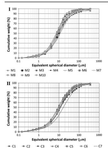
**Fig. 3** Grain-size cumulative curves of the samples collected in Tábua region. I - Monteira group; II - Campelo group
