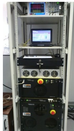
Figure 3.2. HiPIMS-DOMS power supply.
