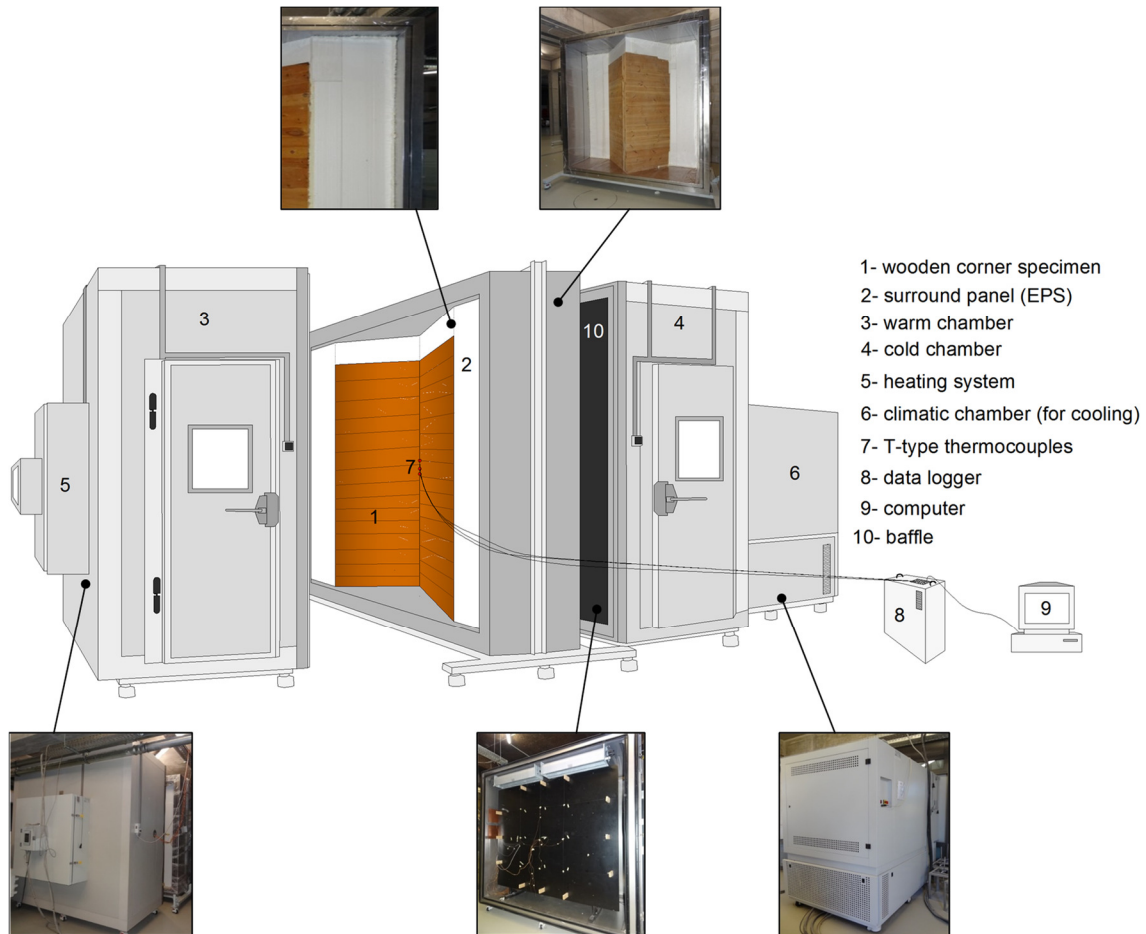
Figure 3.1: Calibrated hot box: apparatus components.
