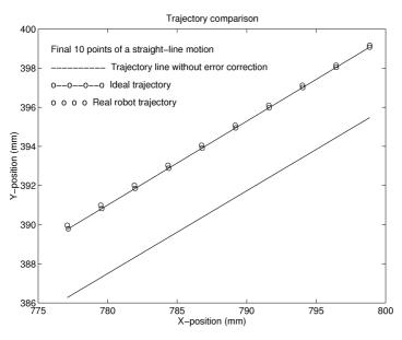
Figure 12. Robot path on the final 10 sampling intervals of motion: ideal trajectory, and trajectories using and not using the algorithm.
