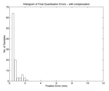
*Figure 14.* Distribution of final-errors on a universe of 100 different straight-line motions using the proposed algorithm. The mean error was m = 0.59 mm with a standard deviation of  $\sigma = 0.49$  mm.
