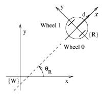
Figure 2. Mobile robot frame and world frame.
