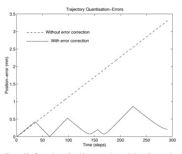
*Figure 11.* Comparison of position-errors time-evolution when moving along one straightline motion. Two situation as are compared: using and not using the algorithm presented in this paper.
