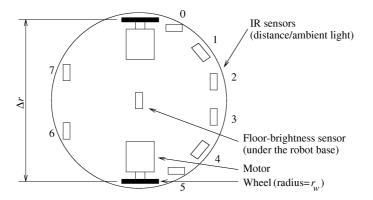
Figure 1. The Khepera miniature mobile robot.
