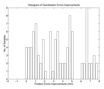
*Figure 15.* Distribution of final-error improvement, obtained on a universe of 100 different straight-line motions, when the proposed algorithm was introduced. The mean improvement was m = 3.49 mm with a standard deviation of  $\sigma = 2.32$  mm.
