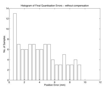
*Figure 13.* Distribution of final-errors on a universe of 100 different straight-line motions that did not use the proposed algorithm. The mean error was m = 4.08 mm with a standard deviation of  $\sigma = 2.59$  mm.
