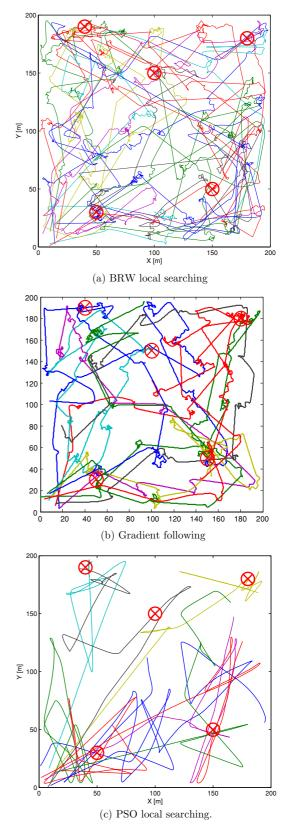
**Fig. 7** Example with the trajectories described by a swarm of 10 robots searching for the source of meandering odour plumes controlled by different local searching strategies
