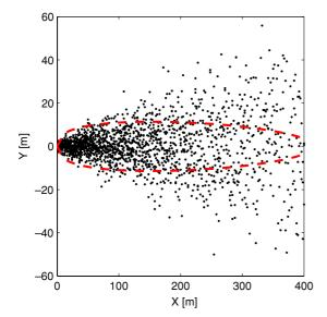
Fig. 1 Concentration at the ground level of a time averaged Gaussian plume generated from a continuous point source localized at ground level in a planar surface. Note that the axis in the figure are not in the same scale
