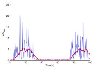
**Fig. 4** Instantaneous concentration measured by a very fast chemical sensor placed in the active area of an odour plume. An electronic nose like the one described shows a response time of about 2 seconds, providing a corresponding low-pass filtered output to the signal represented
