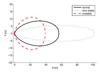
Fig. 6 Active area of the three test plumes used in the simulations. An odour source searching agent will have maximum *detection width* for crosswind movements in stable atmospheres (longer odour plumes).
