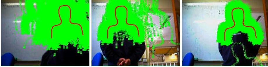
Figure 4.3: Three frames from a head tracking sequence showing the measurement lines of each particle
