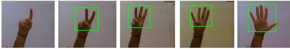
Figure 5.13: Examples of hand detection with bended fingers showing that the occlusion of less than 4 fingers does not affect the performance of the Hand Detection system.
