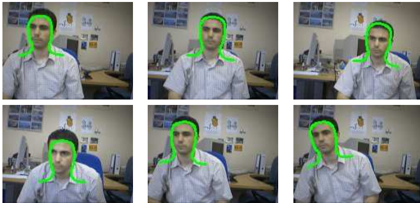
Figure 4.20: Example of tracking a head using combined edges and skin colour classification measures.
