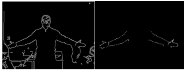
Figure 4.12: Left: all the extracted contours. Right: contours filtered by the optical flow
