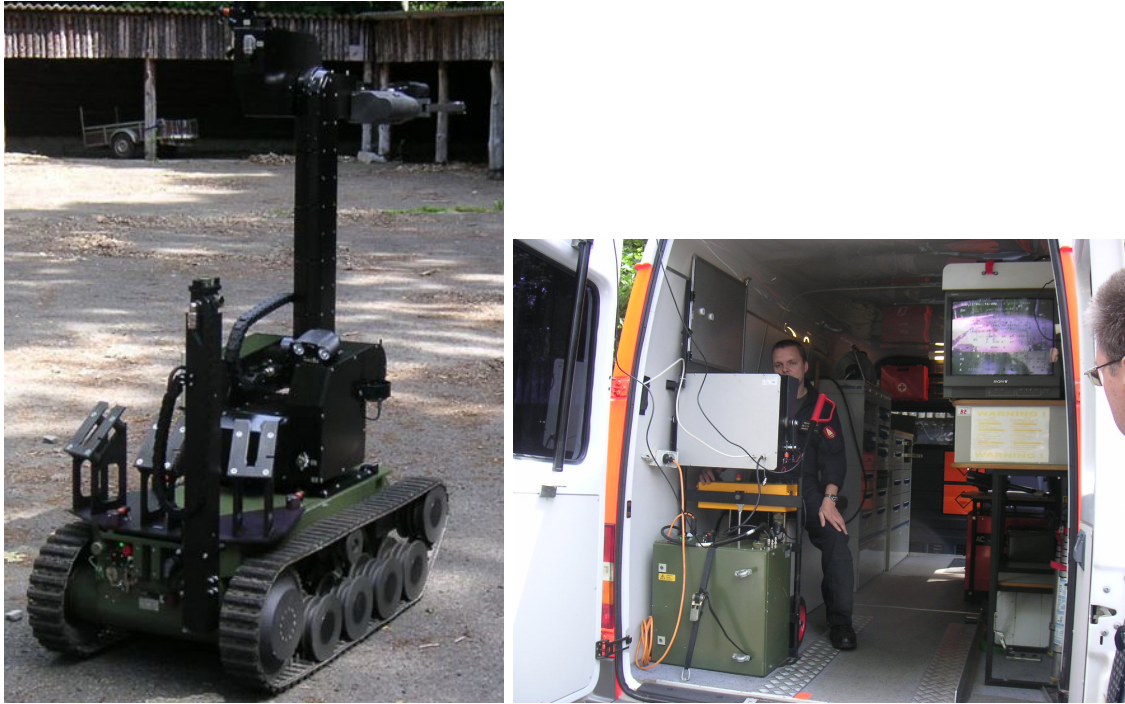
Figure 1.7: A teleoperated robot and its operator panel at Meerdaal Bomb Disposal Unit
