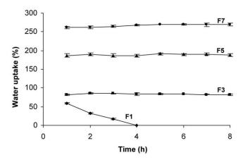
Fig. 3. Graphical representation of the water uptake versus time for several lactose-containing formulations (Table 1) of ketoprofen.
