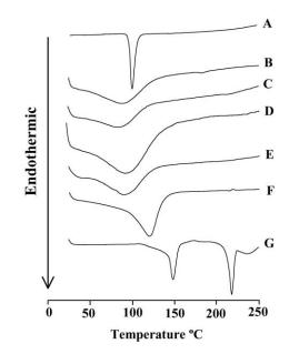
Fig. 1. DSC curves for ketoprofen and the different excipients studied. KETO (A), MC25 (B), HPC (C), HPMC K15M (D), HPMC K100M (E),  $\beta$ -CD (F) and lactose (G).
