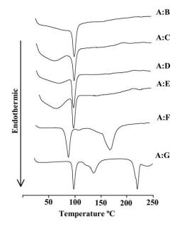
Fig. 2. DSC curves for ketoprofen and 1:1 (w/w) mixtures of ketoprofen with: MC25 (A:B), HPC (A:C), HPMC K15M (A:D), HPMC K100M (A:E),  $\beta$ -CD (A:F) and lactose (A:G).
