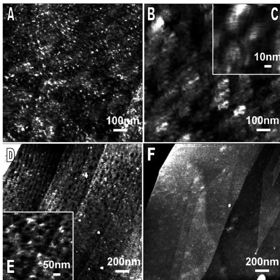
Fig. 1. In situ MAC Mode AFM images in pH 4.50 0.2 M acetate buffer of guanine adsorbed onto HOPG from a saturated guanine solution: (A) after 5 min free adsorption; (B) after 1 h free adsorption; (C) inside image (B). (D) Beginning of dissolution of the guanine layer after one cyclic voltammogram, from 0 to +1.3 V vs. Ag wire, scan rate  $0.05 \text{ V s}^{-1}$ ; (E) inside image (D); (F) complete dissolution of guanine film after performing cyclic voltammetry for 5 min.
