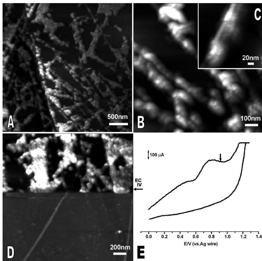
Fig. 2. In situ MAC Mode AFM images in pH 4.50 0.2 M acetate buffer of guanine adsorbed onto HOPG from a saturated guanine solution: (A) after five cyclic voltammograms (CV), from 0 to +1.3 V, scan rate  $100 \text{ mV s}^{-1}$ ; (B) after 5 min at +0.75 V; (C) inside image (B). (D) The applied potential +0.75 V was changed during imaging while running a CV (E) and at  $\sim 0.9 \text{ V}$ , all polymer-like chains were dissolved due to desorption of guanine oxidation products.
