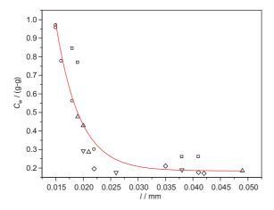
Fig. 6. Effect of thickness, *l*, and cellulose acetate content on the percentage of water uptake ( $C_w$ ), of cellulose acetate/THF membranes, at 25 °C: ( $\Box$ ) CA 1% (wt/v); ( $\bigcirc$ ) CA 5% (wt/v); ( $\triangle$ ) CA 10% (wt/v); ( $\Diamond$ ) CA 15% (wt/v); ( $\bigtriangledown$ ) CA 20% (wt/v).
