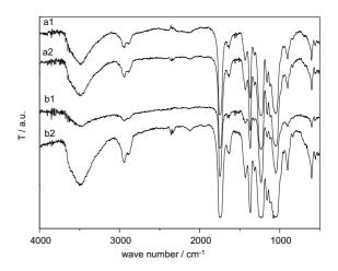
Fig. 2. IR spectra of CA films ( $l = 10 \,\mu\text{m}$ ) prepared using different solvents: acetone (a) and THF (b). Figs. 1 and 2 represent the films dried and in equilibrium with water, respectively.
