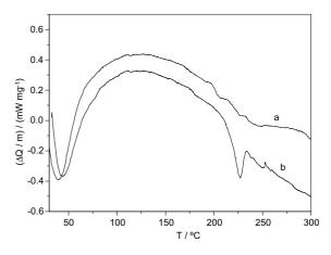
Fig. 3. Differential scanning calorimetry scans of cellulose acetate films with different solvents: (a) THF and (b) acetone. Endothermic transitions are down.
