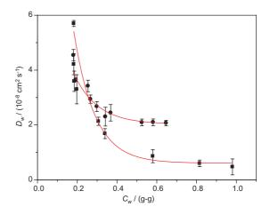
Fig. 8. Effect of weight-weight water concentration,  $C_w$ , on the diffusion coefficient of water,  $D_w$ , in cellulose acetate membranes: ( $\blacksquare$ ) in THF and ( $\bullet$ ) in acetone.
