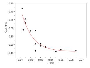
Fig. 7. Effect of thickness, *l*, and cellulose acetate content on the percentage of water uptake ( $C_w$ ), of cellulose acetate/ acetone membranes, at 25 °C: ( $\bullet$ ) CA 5% (wt/v); ( $\blacktriangle$ ) CA 10% (wt/v); ( $\blacklozenge$ ) CA 15% (wt/v).
