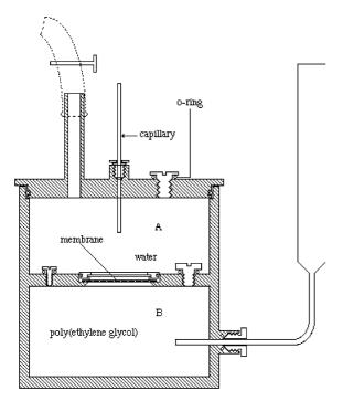
Fig. 1. Schematic representation of the cell developed to measure the integral diffusion coefficients of water in membranes.
