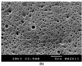
Fig. 5. SEM micrographs of cellulose acetate films prepared with different solvents: (a) acetone, and (b) THF.
