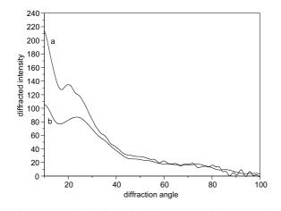
Fig. 4. X-ray diffraction of cellulose acetate films prepared using acetone (a) and THF (b).
