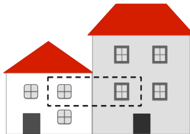
Fig. 7 Complex 3D cadastre occurrences in the medieval Coimbra downtown (Portugal): a flat shared by two buildings.
